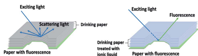
Fig. 9 Schematic diagram for fluorescence to detect the light path of incident light in a multi-layer scattering sample without (left) and with (right) filling with ionic liquid.
