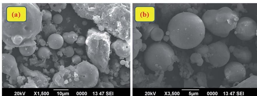
Fig. 3 (a) SEM images of the original fly ash and (b) magnified view of the fly ash.
