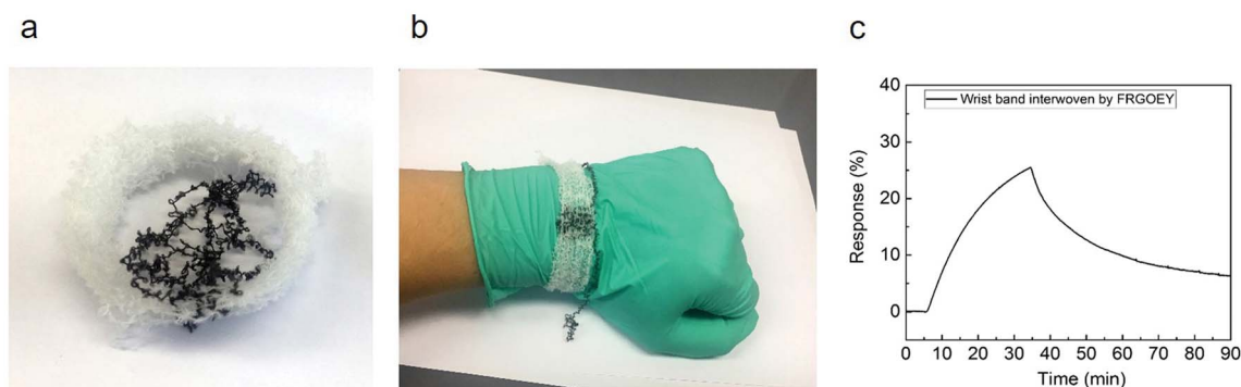
Fig. 5 (a and b) Photographs of the wearable wrist-band integrated with the FRGOEY gas sensor. (c) Response of the wearable gas sensor wrist-band to 500 ppb of NO 2 at room temperature.
