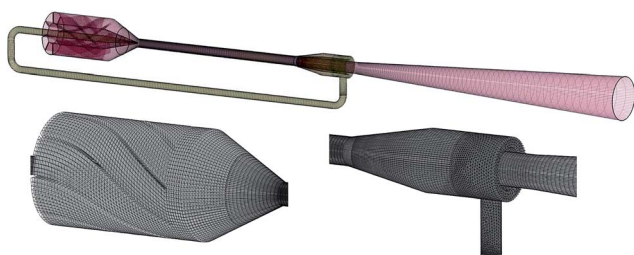
Fig. 3 Mesh methodology for the supersonic separator.
