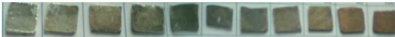
Fig. 1 Photograph showing the various films studied. The compositions from the left are Ag, Ag 0.90 Au 0.10 , Ag 0.80 Au 0.20 , Ag 0.70 Au 0.30 , Ag 0.60 Au 0.40 , Ag 0.50 Au 0.50 , Ag 0.40 Au 0.60 , Ag 0.30 Au 0.70 , Ag 0.20 Au 0.80 , Ag 0.10 Au 0.90 and Au. The colour changes from a metallic grey to dull brown as the Ag content falls.
