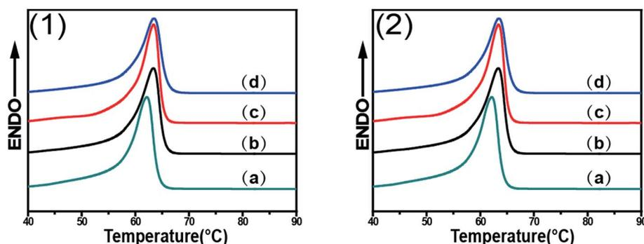
Fig. 7 DSC curves of PCL/0.5 wt% RGO nanocomposites without shear (a) and finishing cooling crystallization with shear at different shear rates (1)  $3 \text{ s}^{-1}$  (2)  $75 \text{ s}^{-1}$  and different shear temperatures (b)  $65 \text{ }^{\circ}\text{C}$ , (c)  $70 \text{ }^{\circ}\text{C}$  and (d)  $75 \text{ }^{\circ}\text{C}$ .
