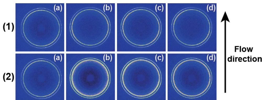
Fig. 1 2D WAXD patterns of PCL/0.5 wt% RGO nanocomposites without shear (a) and finishing cooling crystallization with shear at different shear rates (1) 3 s<sup>-1</sup>, (2) 75 s<sup>-1</sup> and different shear temperatures (b) 65 °C, (c) 70 °C and (d) 75 °C. The flow direction is vertical.
