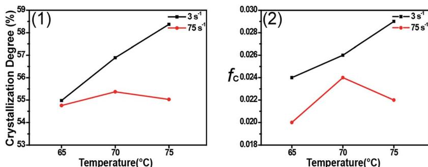
Fig. 3 The crystallinity (1) and the orientation degree of (110) plane (2) of PCL/0.5 wt% RGO nanocomposites finishing cooling crystallization with shear at the shear rates of  $3 \text{ s}^{-1}$  and  $75 \text{ s}^{-1}$  and the shear temperatures of  $65 \text{ }^\circ\text{C}$ ,  $70 \text{ }^\circ\text{C}$  and  $75 \text{ }^\circ\text{C}$ .
