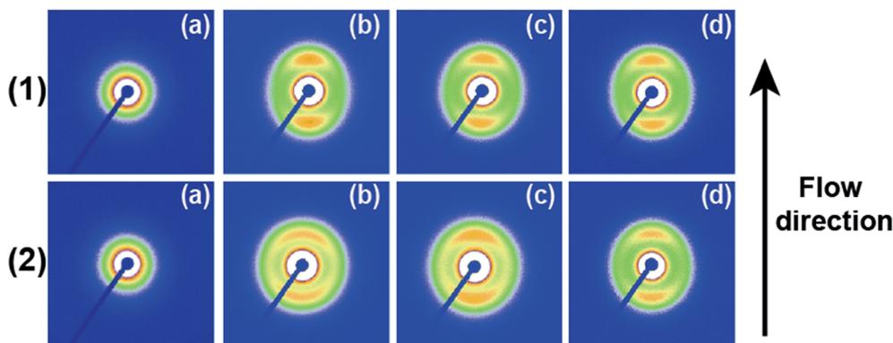
Fig. 4 2D SAXS patterns of PCL/0.5 wt% RGO nanocomposites without shear (a) and finishing cooling crystallization with shear at different shear rates (1)  $3 \text{ s}^{-1}$ , (2)  $75 \text{ s}^{-1}$  and different shear temperatures (b)  $65 \text{ }^\circ\text{C}$ , (c)  $70 \text{ }^\circ\text{C}$  and (d)  $75 \text{ }^\circ\text{C}$ . The flow direction is vertical.
