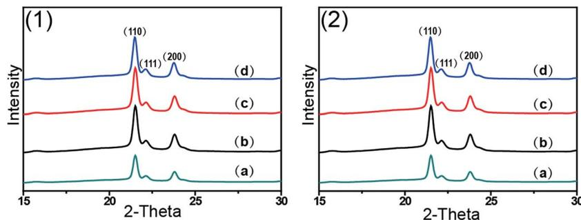
Fig. 2 WAXD curves of PCL/0.5 wt RGO nanocomposites without shear (a) and finishing cooling crystallization with shear at different shear rates (1)  $3 \text{ s}^{-1}$ , (2)  $75 \text{ s}^{-1}$  and different shear temperatures (b)  $65 \text{ }^\circ\text{C}$ , (c)  $70 \text{ }^\circ\text{C}$  and (d)  $75 \text{ }^\circ\text{C}$ .
