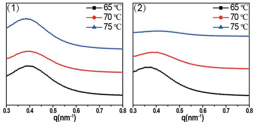
Fig. 6 1D SAXS intensity profile radially integrated of the shear rates (1)  $3 \text{ s}^{-1}$  (2)  $75 \text{ s}^{-1}$  at different shear temperatures of  $65 \text{ }^{\circ}\text{C}$ ,  $70 \text{ }^{\circ}\text{C}$  and  $75 \text{ }^{\circ}\text{C}$ .
