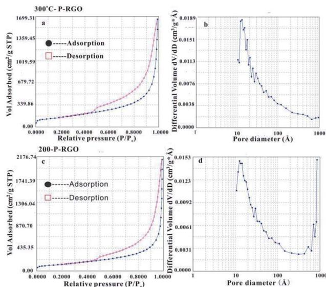
Fig. 5 (a)  $N_2$  physical adsorption isotherm and (b) BJH adsorption pore size distribution of the 300-P-RGO. (c)  $N_2$  physical adsorption isotherm and (d) BJH adsorption pore size distribution of the 200-P-RGO.
