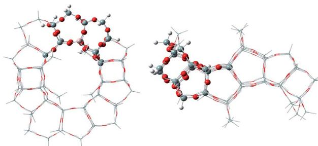
Fig. 1 The 72T ONIOM cluster (the atoms treated with  $\omega\text{B97XD}$  and AM1 are shown in ball and stick modelling and the wireframe, respectively).
