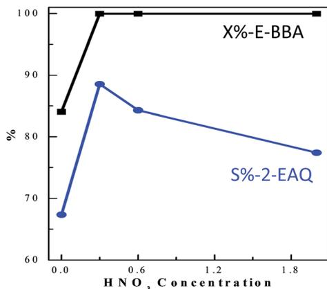
Fig. 11 The effect of HNO<sub>3</sub> treatment on nano-sized H-Beta zeolite in E-BBA dehydration. Reaction conditions: m(E-BBA)/m(Cat) = 1.0, 210 °C, 3.5 h and 0.1 MPa.
