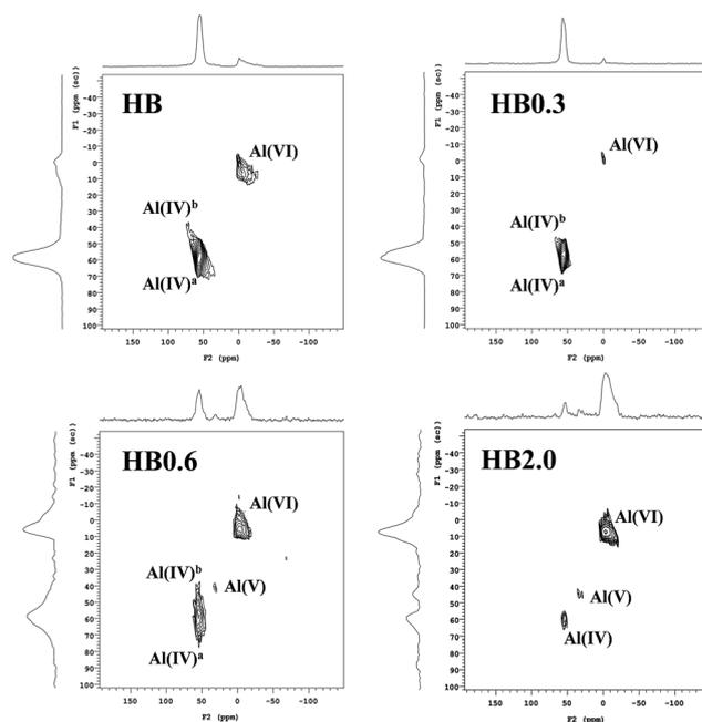
Fig. 4  $^{27}\text{Al}$  MQ MAS NMR spectra of H-Beta and dealuminated H-Beta zeolites. The corresponding  $^{27}\text{Al}$  MAS NMR spectrum is given on top of the MQ MAS plot. The F1 projection shows a purely isotropic dimension, showing a clear resolution of the resonances corresponding to tetrahedral aluminium at different T-positions.
