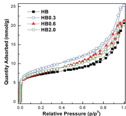
Fig. 6 High-resolution Ar adsorption/desorption isotherms at  $-186\text{ °C}$ .
