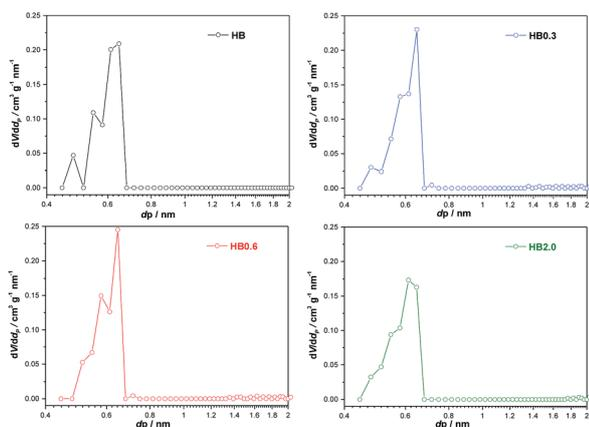
Fig. 7 Pore size distributions of H-Beta and dealuminated H-Beta zeolites obtained by application of the NL-DFT method to the Ar adsorption isotherm at  $-186\text{ }^{\circ}\text{C}$  in the range 0.4–2 nm.
