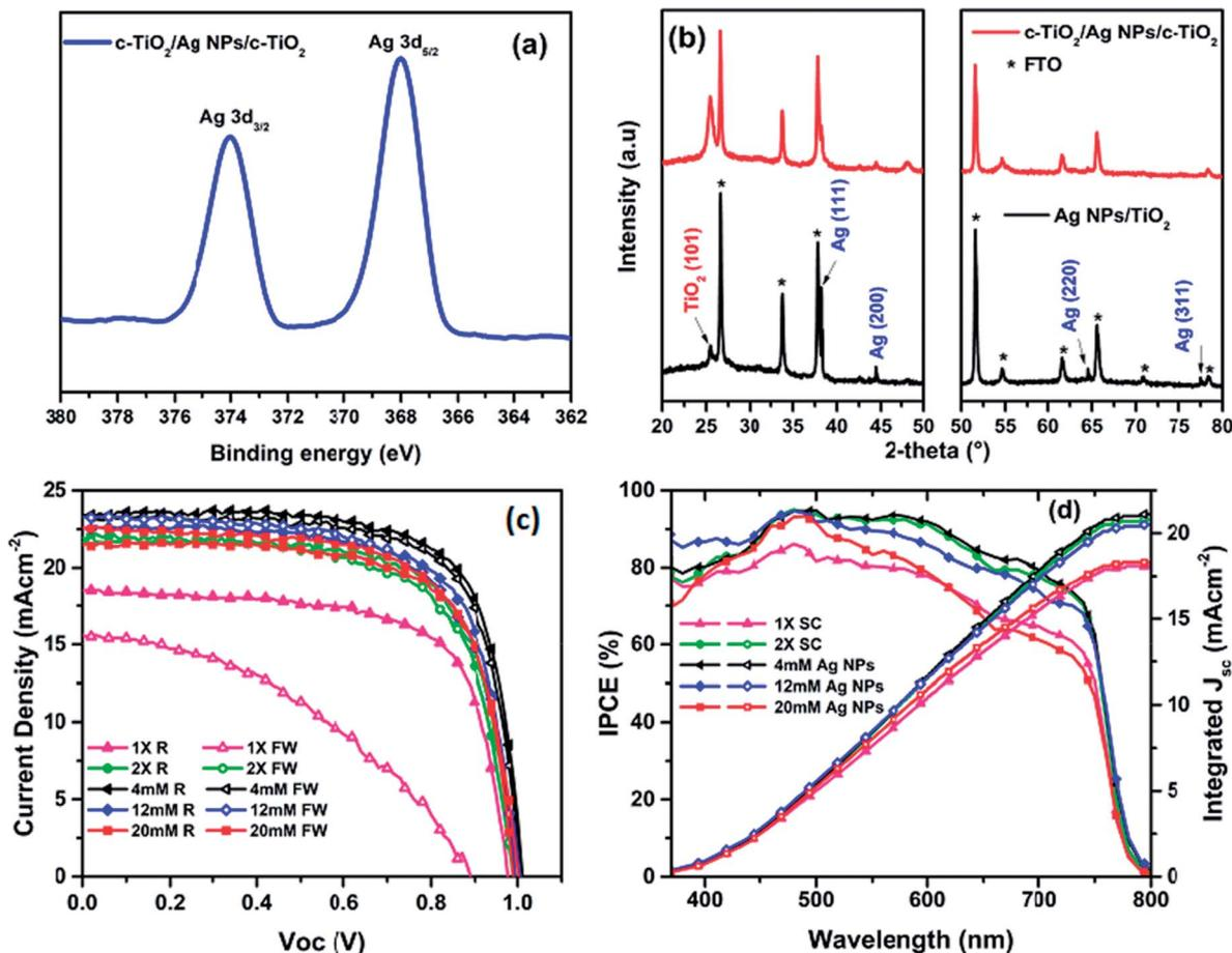
Fig. 1 (a) XPS spectra of  $c\text{-TiO}_2/\text{Ag NPs (4 mM)}/c\text{-TiO}_2$  prepared on FTO substrate (b) XRD of Ag NPs (4 mM)/ $c\text{-TiO}_2$  and  $c\text{-TiO}_2/\text{Ag NPs (4 mM)}/c\text{-TiO}_2$  prepared on FTO. (c) reverse and forward sweep  $J\text{-}V$  characteristics (d) IPCE spectra and integrated  $J_{sc}$  of planar PSCs prepared from control and Ag NPs embedded ETLs.
