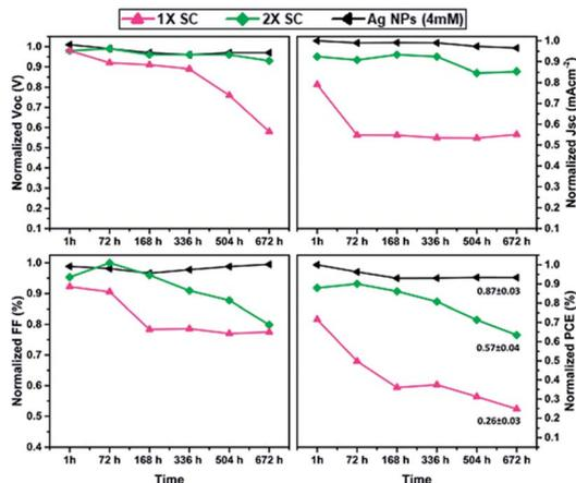
Fig. 6 Long term stability test for 1× SC, 2× SC and Ag NPs (4 mM) ETL based-PSCs without encapsulation for 28 days. The dotted lines represent the maximum values for all device. The standard deviation in the normalized PCE box chart showed the average percentage retained at least for 5 devices.
