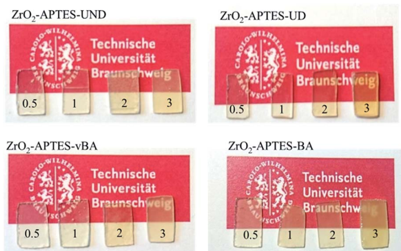
Fig. 10 Photos of cured thin film polystyrene–zirconia NCs filled with different amounts of modified nanoparticles as indicated.
