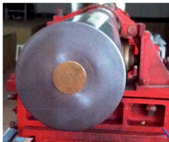
Fig. 3 Pulse shaper used in SHPB apparatus.
