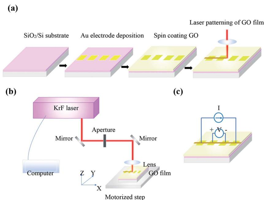
Fig. 1 Schematic of (a) steps proposed to prepare GO films on  $SiO_2/Si$  substrate, (b) KrF laser treatment system of the films and (c) electrical resistance measurements of irradiated films.
