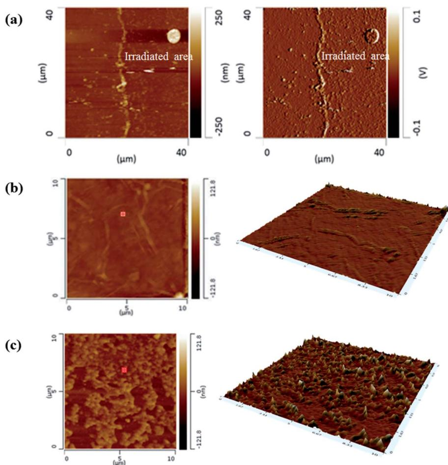
Fig. 2 (a) AFM topography of GO film containing unirradiated and irradiated areas and (b and c) AFM 2D and 3D topography of unirradiated and irradiated areas in a 10 × 10 μm<sup>2</sup> area scan, respectively.
