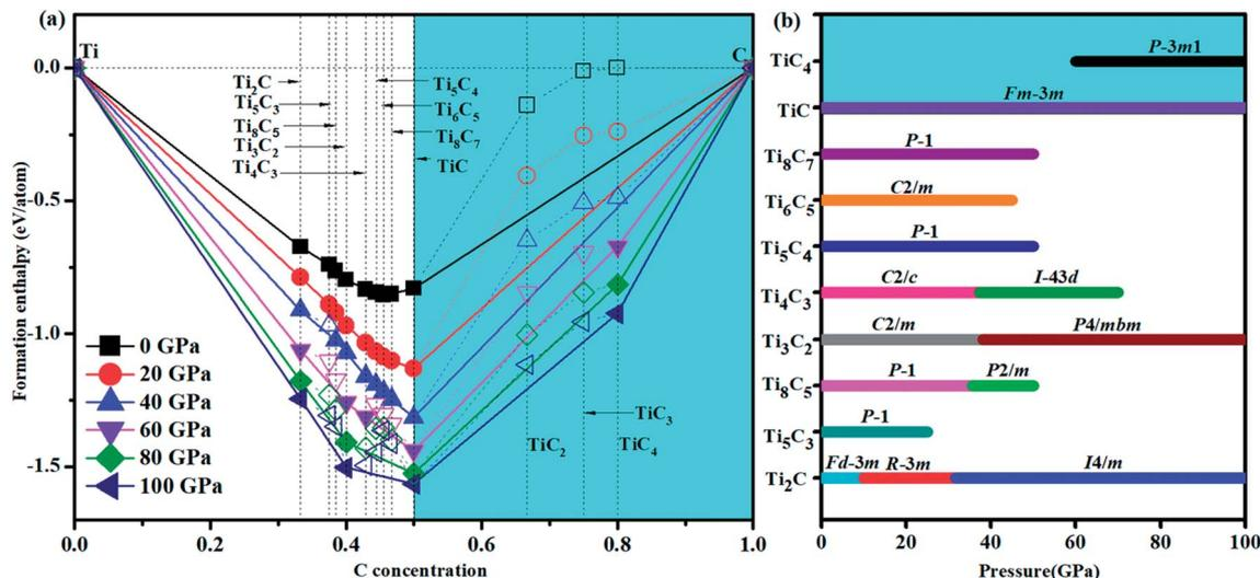
Fig. 1 (a) Convex hull of the Ti–C system. The convex hulls connecting stable phases (solid shapes) are shown by solid lines. Metastable phases (open shapes) are shown by dashed lines. (b) Pressure–composition phase diagram of the Ti–C system. The stable  $TiC_n$  ( $n \geq 1$ ) phases are highlighted by cyan shadows.
