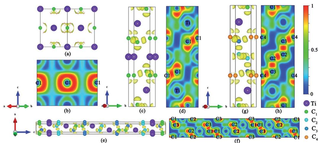
Fig. 6 Calculated ELF of (a) TiC, (b) TiC in the (110) plane, (c) TiC<sub>2</sub>, (d) TiC<sub>2</sub> in the (110) plane, (e) TiC<sub>3</sub>, (f) TiC<sub>3</sub> in the (110) plane, (g) TiC<sub>4</sub>, and (h) TiC<sub>4</sub> in the (110) plane. The calculated ELF isosurface is 0.8.
