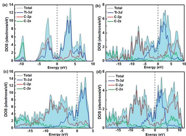
Fig. 4 Calculated total and partial densities of states for (a) TiC, (b) TiC<sub>2</sub>, (c) TiC<sub>3</sub>, and (d) TiC<sub>4</sub>.
