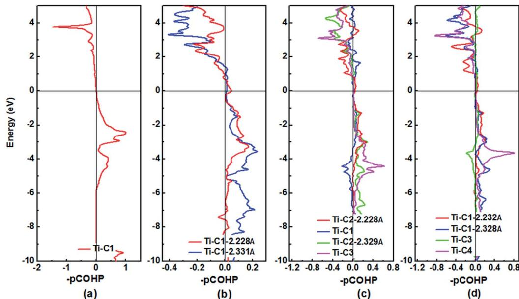
Fig. 5 Plots of the Crystal Orbital Hamilton Population (COHP) for (a) TiC, (b) TiC<sub>2</sub>, (c) TiC<sub>3</sub> and (d) TiC<sub>4</sub> using the pCOHP method. The horizontal line at zero is the Fermi level.
