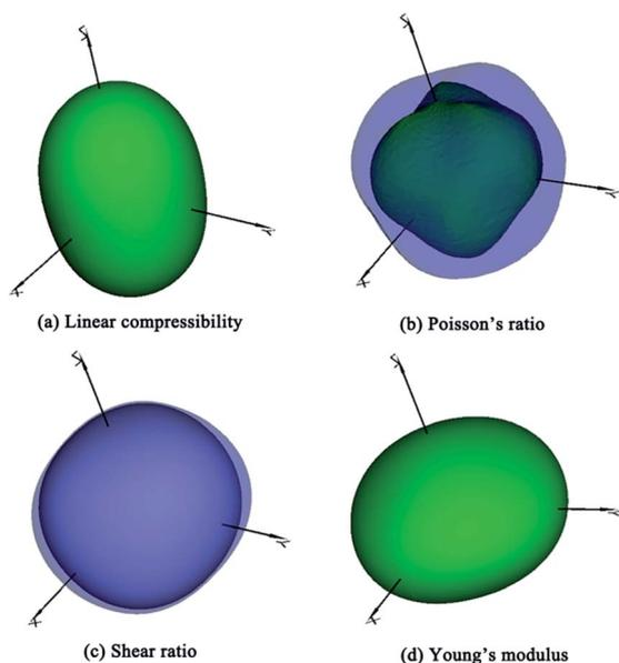
**Fig. 3** The calculated three-dimensional representations of (a) linear compressibility, (b) Poisson's ratio, (c) shear ratio, and (d) Young's modulus for the TiC<sub>2</sub> structure.
