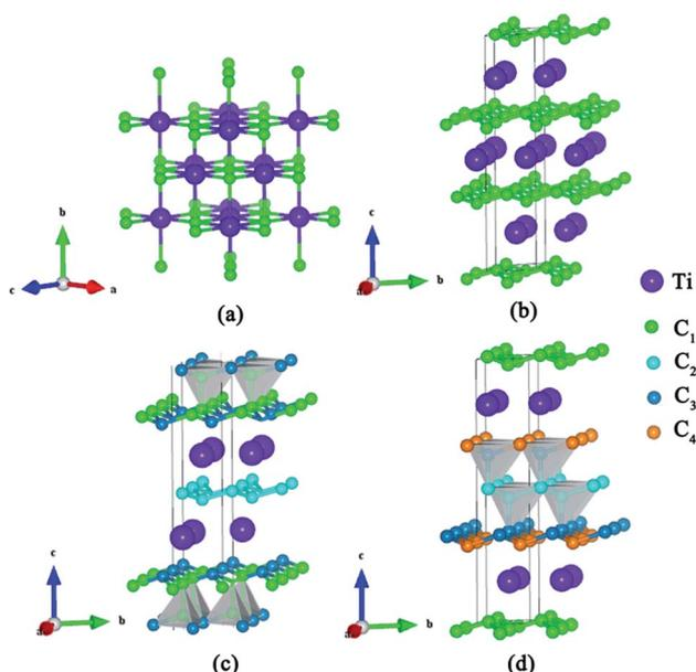
Fig. 2 Crystal structures of titanium carbides. (a)  $TiC$  (SG:  $Fm\bar{3}m$ ), (b)  $TiC_2$  (SG:  $R\bar{3}m$ ), (c) the partial structure of  $TiC_3$  (SG:  $R\bar{3}m$ ) and (d)  $TiC_4$  (SG:  $P\bar{3}m1$ ). The big balls represent titanium atoms, and the small balls represent carbon atoms.
