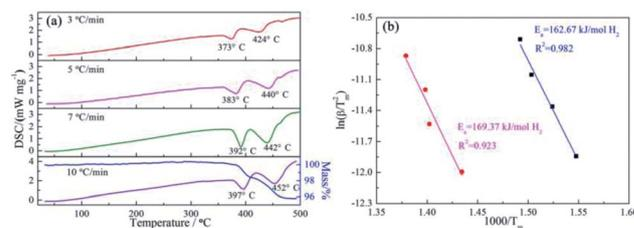
Fig. 1 DSC curves of 3NaBH<sub>4</sub>/ScF<sub>3</sub> composite samples under heating rates of 3 °C min<sup>-1</sup>, 5 °C min<sup>-1</sup>, 7 °C min<sup>-1</sup> and 10 °C min<sup>-1</sup> and TG profile at the heating rate of 10 °C min<sup>-1</sup> (a) and the corresponding Kissinger plots for the two major endothermic desorption steps (b).
