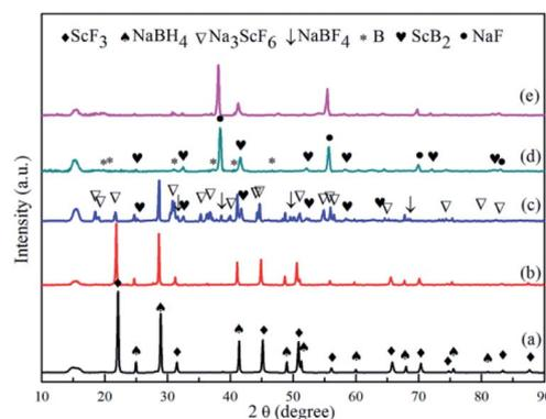
**Fig. 3** XRD patterns of the  $3\text{NaBH}_4/\text{ScF}_3$  composite after ball milling (a), dehydrogenated at  $300 \text{ }^\circ\text{C}$  (b), dehydrogenated at  $420 \text{ }^\circ\text{C}$  (c), fully dehydrogenated at  $530 \text{ }^\circ\text{C}$  (d) and rehydrogenated at  $420 \text{ }^\circ\text{C}$  (e).
