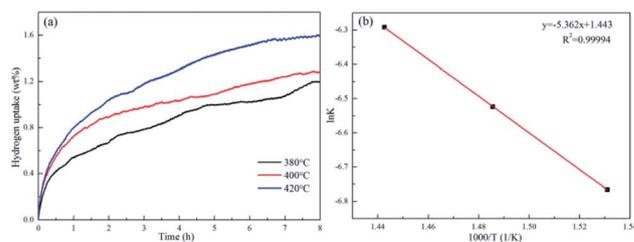
Fig. 5 Isothermal hydrogen absorption curves for the partially dehydrogenated  $3\text{NaBH}_4/\text{ScF}_3$  composite sample at temperatures of  $380\text{ }^\circ\text{C}$ ,  $400\text{ }^\circ\text{C}$  and  $420\text{ }^\circ\text{C}$  (a) and the  $\ln k - 1000/T$  fitting plot (b).
