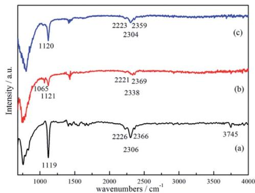
Fig. 7 FTIR spectra of the  $3\text{NaBH}_4/\text{ScF}_3$  composite after ball-milling (a), half dehydrogenated  $3\text{NaBH}_4/\text{ScF}_3$  sample (b), rehydrogenation of partially dehydrogenated  $3\text{NaBH}_4/\text{ScF}_3$  sample (c).
