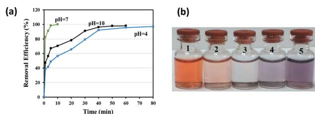
Fig. 5 (a) The effect of initial solution pH of CR on removal efficiency. (b) The photos of 1: CR solution (20.0 mg L<sup>-1</sup>) at natural or basic pH; 2, 3 and 4: CR solution (20.0 mg L<sup>-1</sup>) treated with 15.0 mg aerogel after 10 min at pH 10.0, 7.0 and 4.0, respectively and 5: CR solution (20.0 mg L<sup>-1</sup>) at acidic pH.
