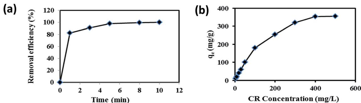
Fig. 7 (a) Effect of contact time on the adsorption capacity (CR solution: 20.0 mg L<sup>-1</sup>, pH 7.0, adsorbent dose: 0.015 g/30.0 mL). (b) Effect of CR concentration on the adsorption capacity (pH 7.0, adsorbent dose: 0.015 g/30.0 mL).
