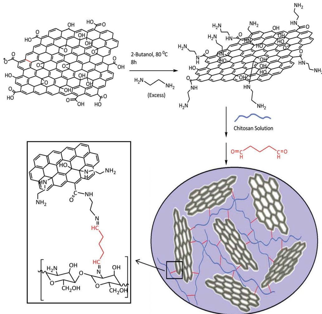
Scheme 1 Synthetic route of GN-CS nanocomposite hydrogel.
