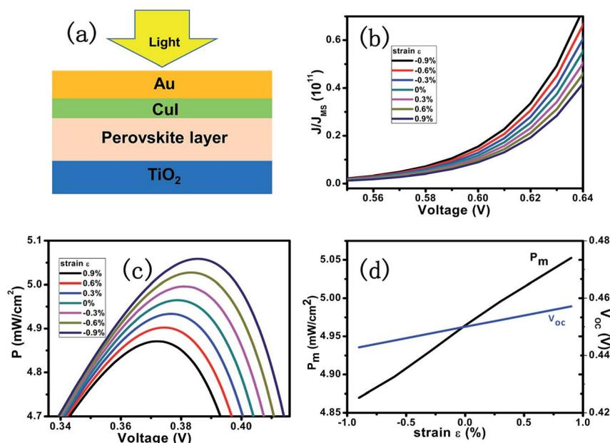
Fig. 2 (a) Schematic of a PPSC with  $\text{CH}_3\text{NH}_3\text{PbI}_3$  thin film sandwiched between  $\text{CuI}$  and  $\text{TiO}_2$ . (b) Relative current density varying with voltage when applied compressive strains ranging from  $-0.9\%$  to  $0.9\%$  applied. (c) Output power of a PPSC as a function of voltage with various strains applied. (d) Maximum output power and open-circuit voltage under various compressive strains.
