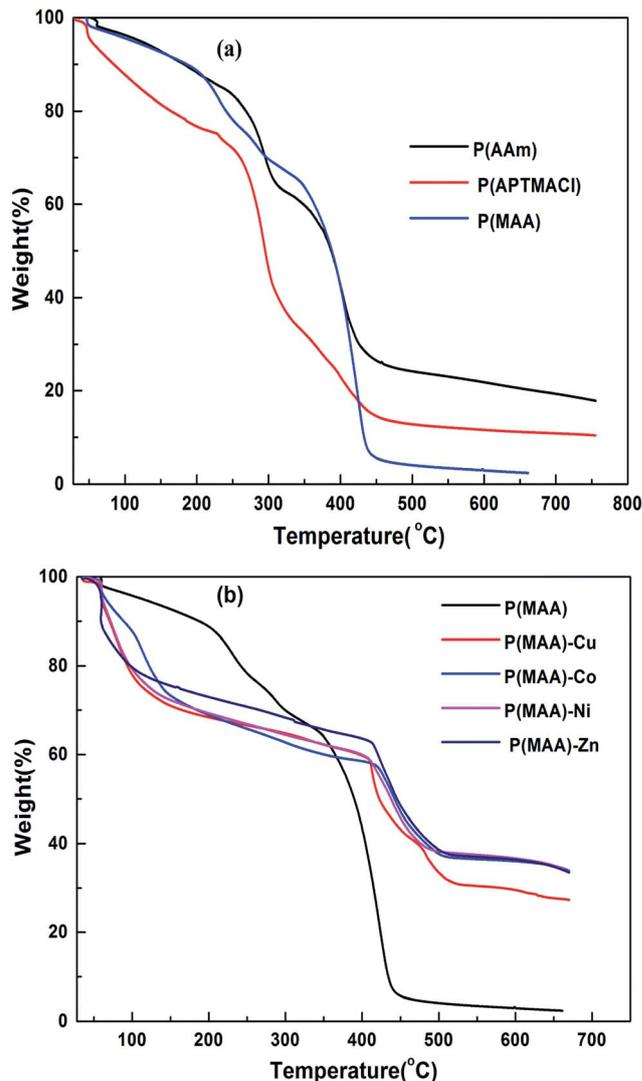
Fig. 4 TGA curves for (a) pure hydrogels and (b) P(MAA) pure and metal entrapped hybrid hydrogels.
