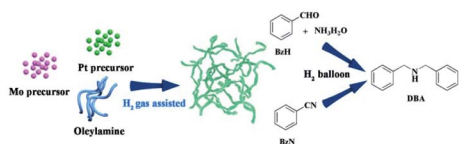
Scheme 1 Schematic of the synthesis of PtMo WNWs and its catalytic application in the DBA synthesis from reductive amination of either BzH or BzN.
