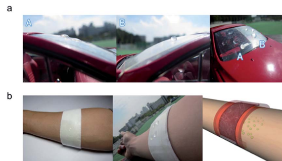
Fig. 12 Promising applications of PTFE/Ag NW/PET and PTFE/Ag NW/PU samples. (a) Transparent TFHs attached to the curved window of an automobile can be used as a defogging and deicing system. PTFE/Ag NW/PET based flexible TFH sample was attached to the self-cleaning window of the automobile. The A region is the bare Ag NW electrode and the B region is the PTFE/Ag NW electrode. (b) The stretchable TFHs attached to medical patches enhanced drug diffusion through the skin. The hydrophobic properties of the PTFE/Ag NW/PU based stretchable TFHs led to a waterproof effect.
