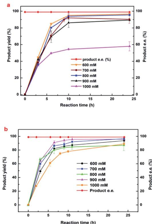
Fig. 5 The effects of (a) histidine and (b) His–Na<sub>2</sub>CO<sub>3</sub> composite regulating method on the synthesis of (*R*)-HBME. Reaction conditions: 1000 mM glucose, 60 mg mL<sup>-1</sup> microbial cells (wet weight), 4 mL phosphate buffer (200 mM, pH 7.0), 200 rpm, 40 °C, MAA of the designated concentration. Tuning pH of the reaction mixture to approximately 6.5 and 7.0 every 3 h by His and His–Na<sub>2</sub>CO<sub>3</sub>, respectively.
