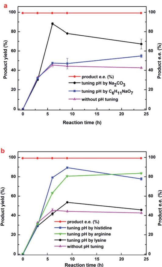
Fig. 4 The effects of variable alkaline compound regulating method on the synthesis of (*R*)-HBME. Reaction conditions: 450 mM MAA, 60 mg mL<sup>-1</sup> microbial cells (wet weight), 1000 mM glucose, 4 mL phosphate buffer (200 mM, pH 7.0), 200 rpm, 35 °C. Tuning pH of the reaction mixture by different alkaline compounds.
