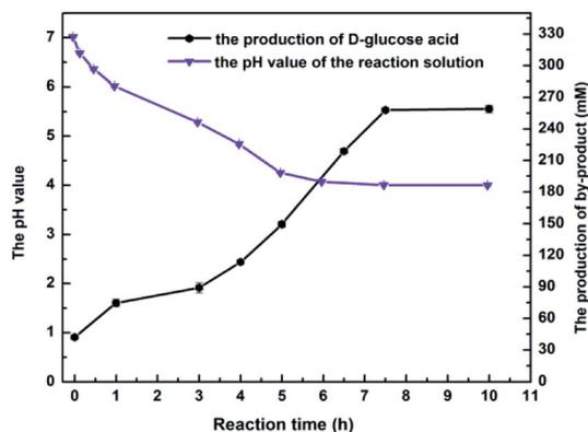
Fig. 3 The online monitoring of pH and *D*-glucuronic acid in the course of the reaction. Reaction conditions: 350 mM MAA, 800 mM glucose, 60 mg mL<sup>-1</sup> microbial cells (wet weight), 4 mL phosphate buffer (200 mM, pH 7.0), 200 rpm, 40 °C.
