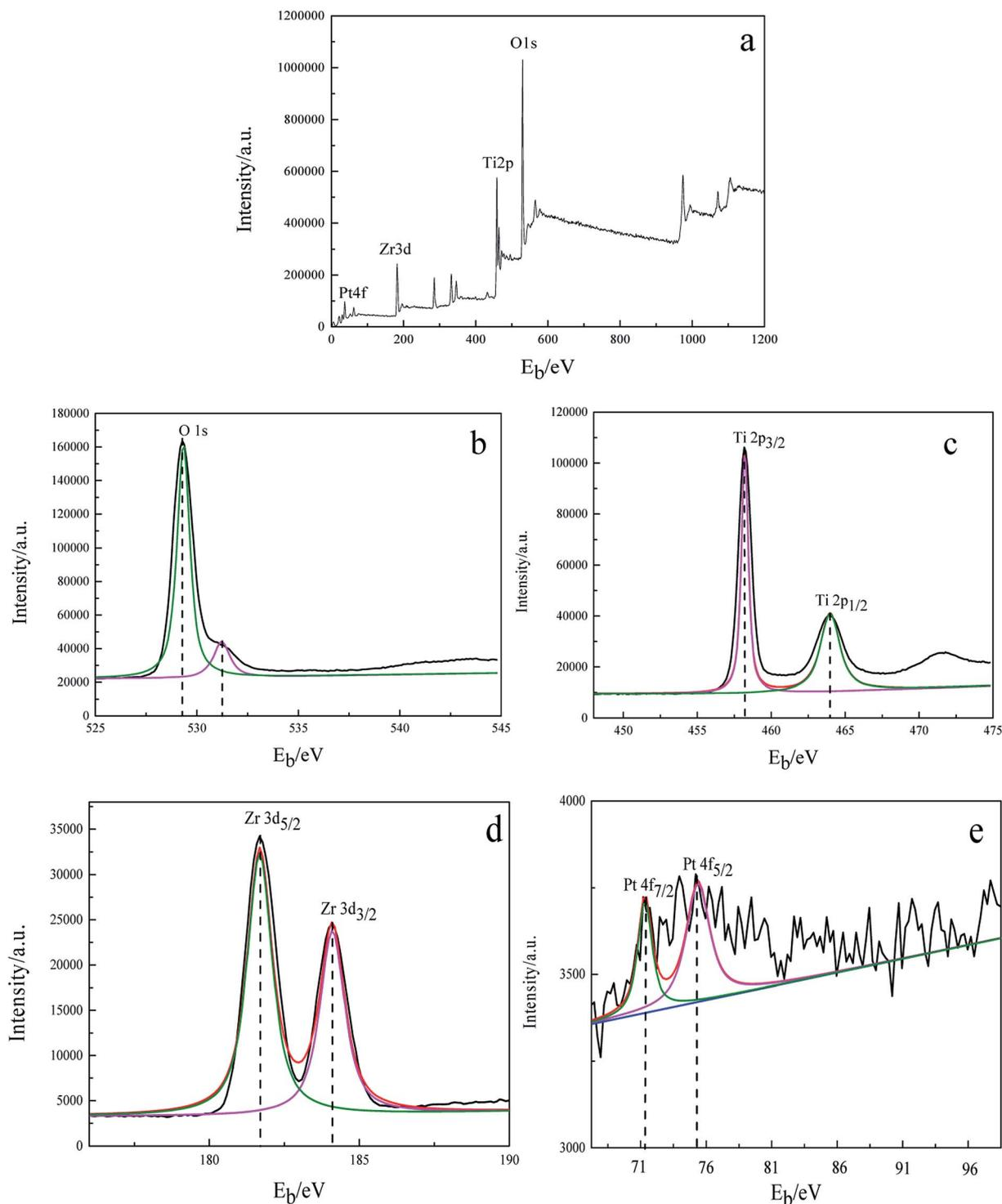
Fig. 3 X-ray photoelectron spectra of 3DOM Pt/TiO<sub>2</sub>-ZrO<sub>2</sub>. (a) Full spectrum; (b) O 1s; (c) Ti 2p; (d) Zr 3d; and (e) Pt 4f.
