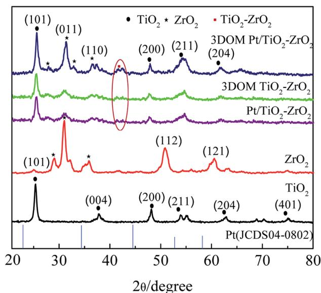
Fig. 1 X-ray diffraction patterns of different materials.
