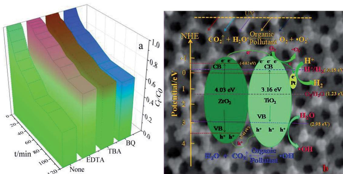
Fig. 8 UV photocatalytic degradation of MG with different trapping agents (a) and possible photocatalytic reaction mechanism of 3DOM Pt/TiO<sub>2</sub>-ZrO<sub>2</sub> (b).
