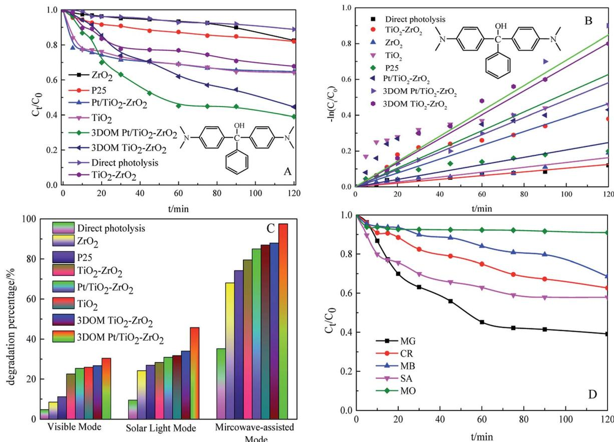
Fig. 6 Photodegradation of malachite green with different catalysts under UV light irradiation (A), kinetics diagram of different catalysts for the degradation of malachite green (B), photodegradation of malachite green with different catalysts under simulated sunlight and microwave-assisted irradiation (C), and results of photodegradation of different dyes by 3DOM Pt/TiO<sub>2</sub>-ZrO<sub>2</sub> (D).
