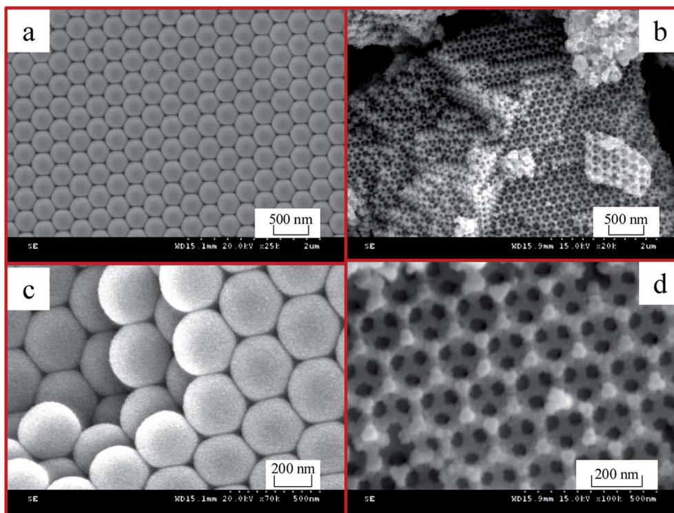
Fig. 4 SEM images of polystyrene (PS) microspheres (a and c) and 3DOM Pt/TiO<sub>2</sub>-ZrO<sub>2</sub> (b and d).
