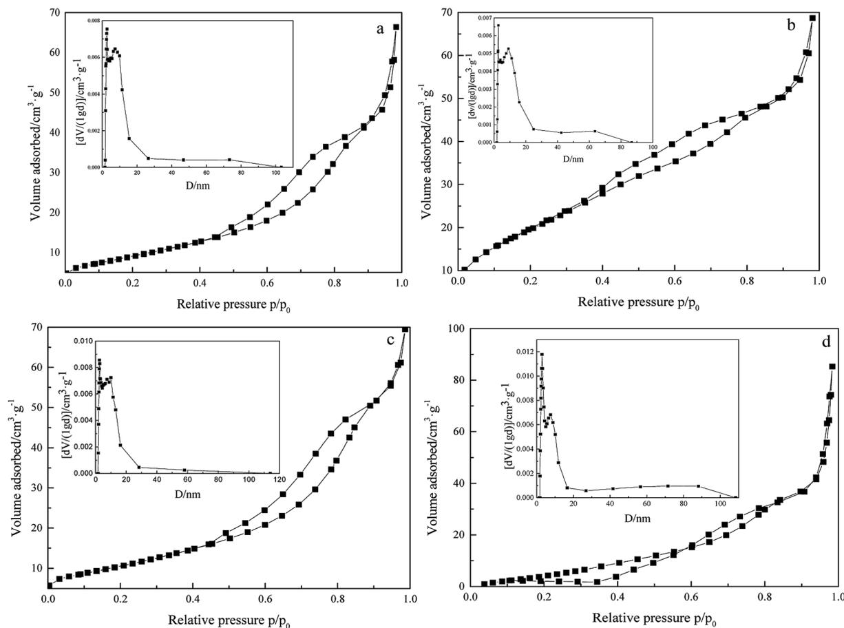
Fig. 5  $N_2$  adsorption–desorption isotherms of 3DOM Pt/TiO<sub>2</sub>–ZrO<sub>2</sub> (a), Pt/TiO<sub>2</sub>–ZrO<sub>2</sub> (b), 3DOM TiO<sub>2</sub>–ZrO<sub>2</sub> (c), and TiO<sub>2</sub>–ZrO<sub>2</sub> (d) (insets show the BJH pore size distribution curves).
