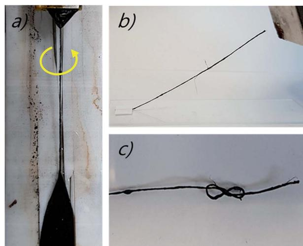
Fig. 2 (a) Optical images showing the magnetic ribbon-shaped MWNT sheet is being fabricated by the biscrolling method,<sup>1</sup> (b) the attraction of the magnet yarn to a magnet, and (c) a knotted magnetic-particle-filled MWNT yarn.
