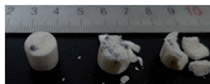
Fig. 11 Typical fragments collected after quasi-static tests at 50 °C, 75 °C and 100 °C.
