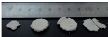
Fig. 13 Typical fragments collected after dynamic compression at 15 °C, 50 °C, 75 °C and 100 °C.
