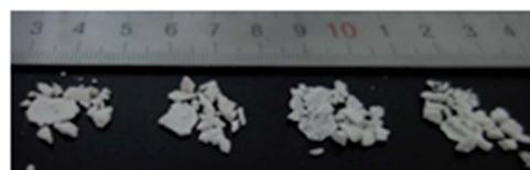
Fig. 12 Typical fragments collected after dynamic compression at -25 °C, -50 °C, -75 °C and -100 °C.
