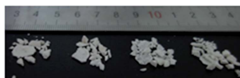
Fig. 12 Typical fragments collected after dynamic compression at -25 °C, -50 °C, -75 °C and -100 °C.
