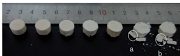
Fig. 9 Typical fragments collected at 15 °C (room temperature), 0 °C, -25 °C, -50 °C, -75 °C, -100 °C and -125 °C.
