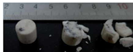
Fig. 11 Typical fragments collected after quasi-static tests at 50 °C, 75 °C and 100 °C.
