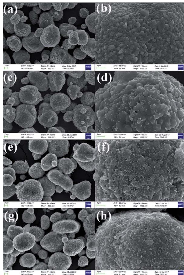
Fig. 3 SEM images of (a and b) the pristine  $\text{LiMn}_2\text{O}_4$ , (c and d) 1 wt%, (e and f) 3 wt%, and (g and h) 5 wt%  $\text{ZrO}_2$ -coated  $\text{LiMn}_2\text{O}_4$  obtained by calcining 0, 1.19, 3.56, and 5.93 wt%  $\text{ZrO}_2$ -coated  $\text{Mn}_3\text{O}_4$  &  $\text{Li}_2\text{CO}_3$  mixtures at 800 °C for 20 h.
