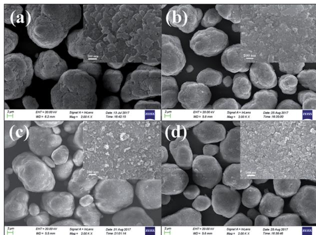
Fig. 2 SEM images of (a) the pristine  $\text{Mn}_3\text{O}_4$  and (b) 1.19 wt%, (c) 3.56 wt%, (d) 5.93 wt%  $\text{ZrO}_2$ -coated  $\text{Mn}_3\text{O}_4$  without any heat-treatment. The insets are the corresponding SEM images at high magnification.
