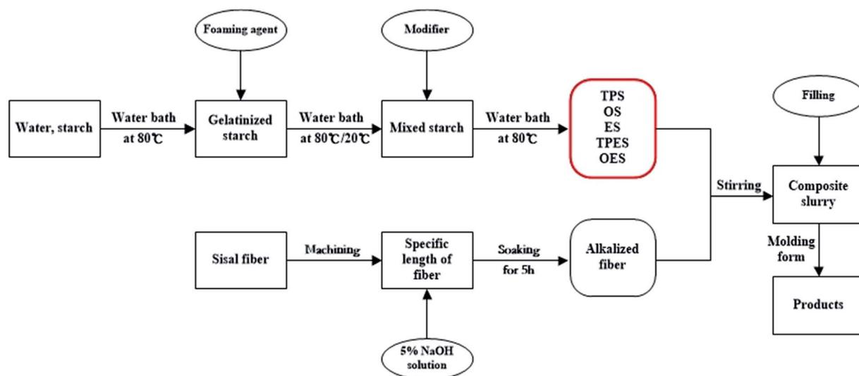
Fig. 1 Flow chart of the preparation of starch-based composites.
