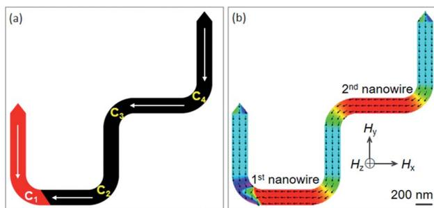
Fig. 14 (a) A DWT structure was designed with  $\beta = 90^\circ$ . (b) An OOMMF image of the  $90^\circ$ -DWT, at which a TDW was created at the  $C_1$  corner of the structure. Herein, the four corners ( $C_{1-4}$ ) of the structure were smoothed to assist a DW which can easily propagate through the structure using the two-field directions.
