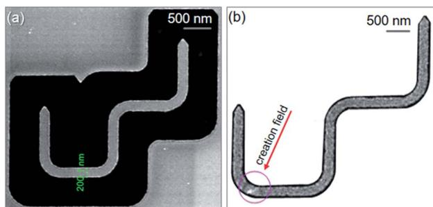
Fig. 16 (a) A SEM image of the 90°-DWT structure which was designed, as given in Fig. 14(a), and patterned using the FIB method.<sup>29</sup> (b) A Fresnel image of the patterned structure where a CW-VDW was created at the  $C_1$  corner using the creation field strength of 0.5 T with  $\alpha \approx 30^\circ$ .
