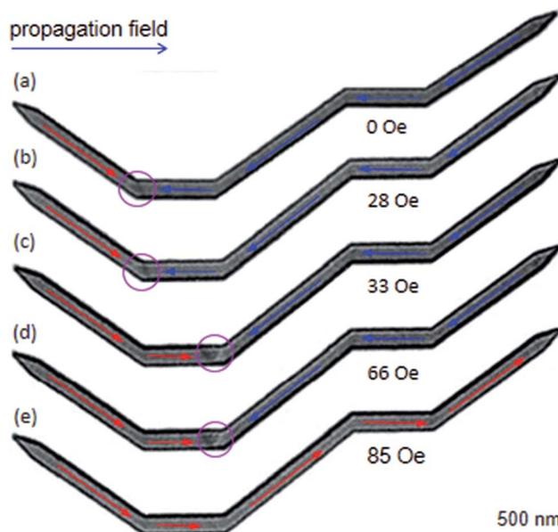
Fig. 7 Lorentz images of the modified DWT structure where the diamond pads of the structure were modified in either side. (a) A TDW was created at the  $C_1$  corner of the structure with the creation field strength of 0.5 T ( $\alpha = 40^\circ$ ). (b)–(d) The created TDW was propagated from the  $C_1$  to  $C_2$  corner with increments of the propagation field. (e) The TDW was removed out the structure at the field strength of 85 Oe.
