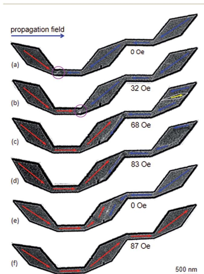
Fig. 5 Lorentz images of the original DWT structure: (a) a CW-VDW was created by an external field of 0.5 T, the field was applied with an oblique angle of  $\approx 40^\circ$  ( $\alpha$ ), as also given in Fig. 4(a). (b) A Lorentz image of the DWT structure when the propagation field of 32 Oe was applied. (c)–(f) Lorentz images of the DWT structure which were recorded at various field strengths.
