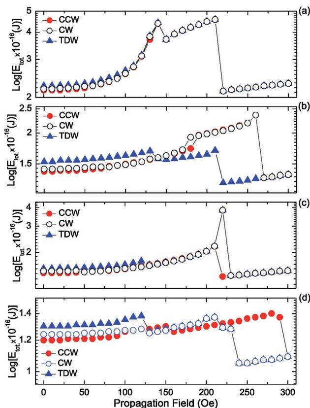
Fig. 9 Total energies of the DWs created at the  $C_1$  corners of the DWT structures as a function of propagation fields, for the structures (a) without, (b) upper, (c) lower and (d) with either-side diamond-pad modifications. Therein, the red-solid-circle ( $\bullet$ ), black-open-circle ( $\circ$ ) and blue-solid-triangle ( $\blacktriangle$ ) symbols represent the total energies of the CCW-VDW, CW-VDW and TDW, respectively.
