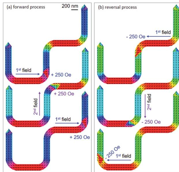
Fig. 15 OOMMF images of (a) forward and (b) reversal processes of a TDW which was created, and propagated through the  $90^\circ$ -DWT structure ( $\beta = 90^\circ$ ) using the two-field directions. The field strength requires for each sequence is equal to 250 Oe.
