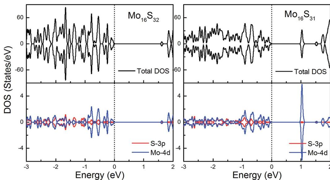
Fig. 6 Total DOS and partial DOS for pristine 1H-MoS<sub>2</sub> with and without S vacancies. The dashed line indicates the Fermi level at 0 eV.
