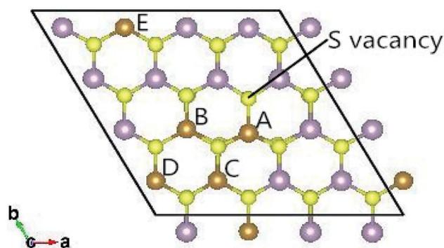
Fig. 1 Top view of the  $4 \times 4 \times 1$  supercell of the defective 1H-MoS<sub>2</sub> impurities. Five configurations are taken into account in this work and marked as Mo<sub>15</sub>XS<sub>31</sub>-A, B, C, D, or E according to the distance between the dopant and S vacancy.
