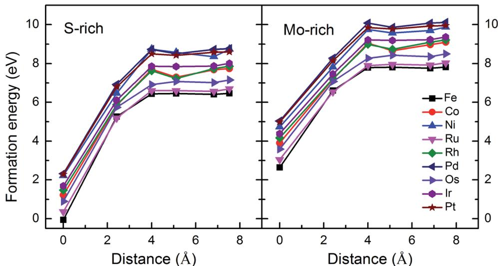
Fig. 2 Formation energies as a function of the distance between the S vacancy and impurity atoms in S-rich and Mo-rich conditions.
