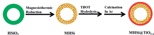
Fig. 1 Schematic illustration for the synthesis of MHSi@TiO 2-x composite.
