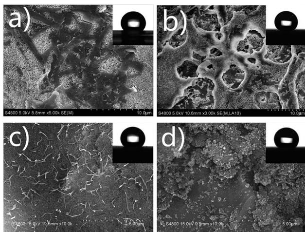
Fig. 3 SEM images of coatings prepared in different conditions. (a) Cooled to 25 °C, (b) without cooling process, (c) cooling with stirring, (d) dried at 80 °C for 5 min.
