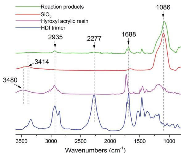
Fig. 1 FTIR spectra of HDI trimer, hydroxyl acrylic resin, SiO<sub>2</sub> and reaction products.
