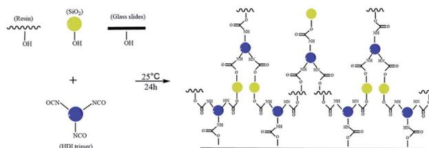
Scheme 1 Possible bonding structures among SiO<sub>2</sub>, hydroxyl acrylic resin and HDI trimer on glass slides.
