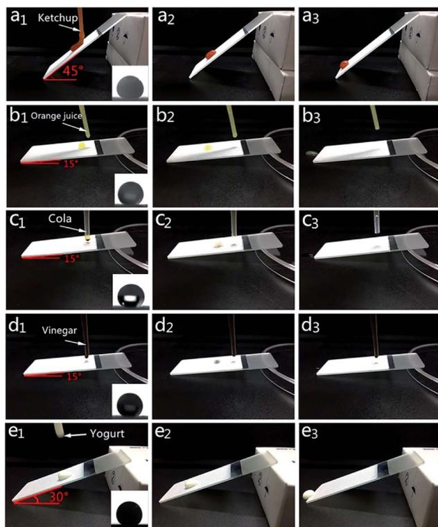
Fig. 6 Rolling processes of ketchup (a<sub>1</sub>–a<sub>3</sub>), orange juice (b<sub>1</sub>–b<sub>3</sub>), cola (c<sub>1</sub>–c<sub>3</sub>), vinegar (d<sub>1</sub>–d<sub>3</sub>), yogurt (e<sub>1</sub>–e<sub>3</sub>) on the coated surfaces.
