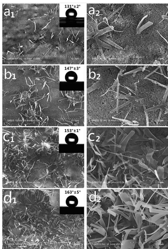
Fig. 2 SEM images of micro-nanoscale structures of SPEW coatings with various PEW dosages. (a<sub>1</sub>) 10 wt%, (b<sub>1</sub>) 15 wt%, (c<sub>1</sub>) 20 wt%, (d<sub>1</sub>) 25 wt%; (a<sub>2</sub>–d<sub>2</sub>) expansion images from (a<sub>1</sub>–d<sub>1</sub>).
