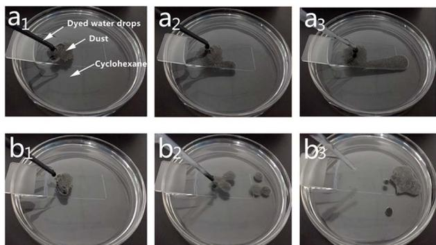
Fig. 7 Self-cleaning test on uncoated surface (a<sub>1</sub>–a<sub>3</sub>) and coated surface (b<sub>1</sub>–b<sub>3</sub>) when surfaces immersed in cyclohexane.
