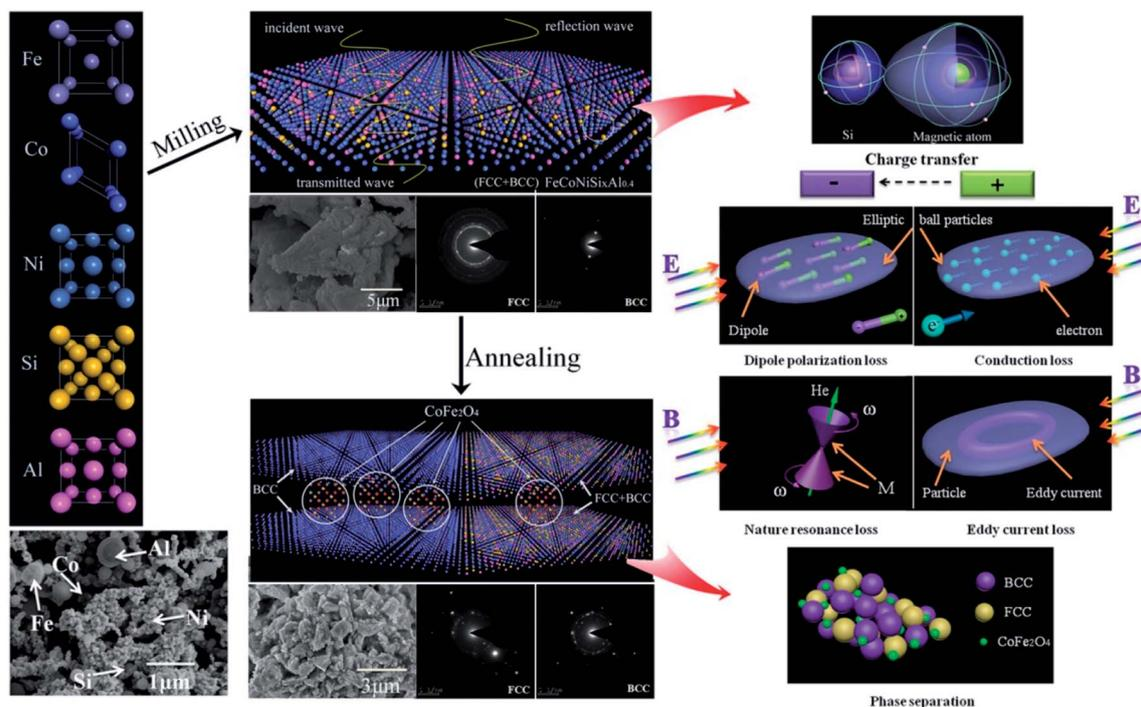
Fig. 7 Schematic illustration of the change of crystal structure in the process of milling and annealing and the mechanism interacted with EM wave for HEA powders.
