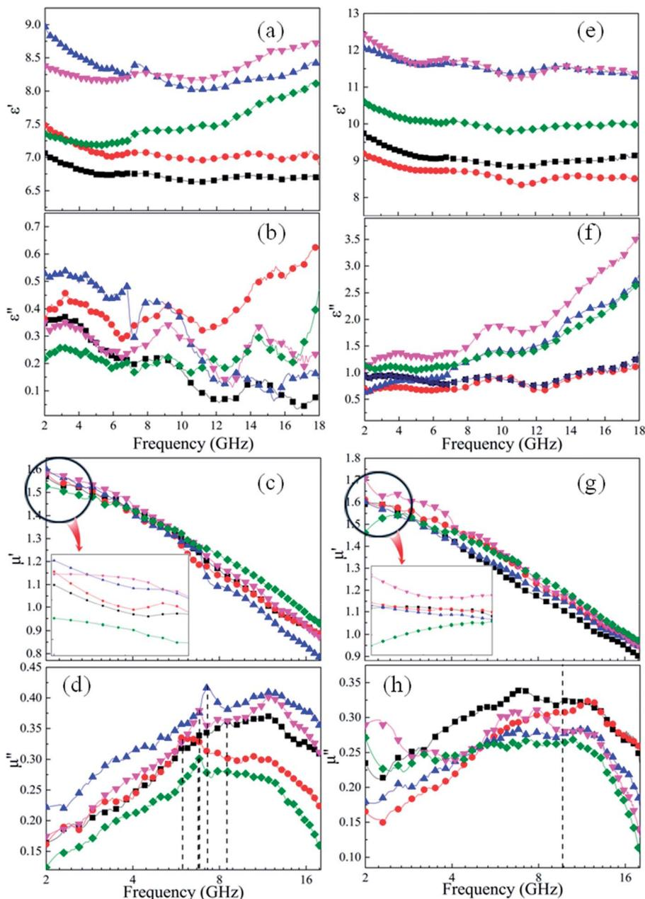
Fig. 5 Frequency dependence of (a and e)  $\epsilon'$ , (b and f)  $\epsilon''$ , (c and g)  $\mu'$ , and (d and h)  $\mu''$  for the (a–d) as-milled and (e–h) as-annealed  $\text{FeCoNiSi}_x\text{Al}_{0.4-x}$ –paraffin composites. The symbols of  $\blacksquare$ ,  $\bullet$ ,  $\blacktriangle$ ,  $\blacktriangledown$  and  $\blacklozenge$  denote the  $x = 0.1, 0.2, 0.3, 0.4$ , and  $0.5$  composites, respectively.
