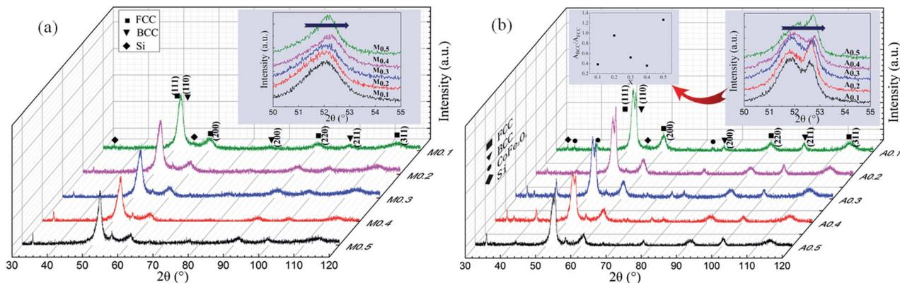
Fig. 1 XRD patterns of (a) as-milled and (b) as-annealed  $\text{FeCoNiSi}_x\text{Al}_{0.4}$  HEA powders, and the detailed scans in the range of  $2\theta = 50\text{--}55^\circ$  are presented in the illustration. The change in area ratio ( $A_{\text{BCC}}/A_{\text{FCC}}$ ) for the as-annealed HEA powders is also presented in the illustration. All alloys are composed of BCC and FCC phase except a small amount of Si remained indicating the formation of high entropy alloy.
