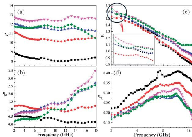
Fig. 9 Frequency dependence of (a)  $\epsilon'$ , (b)  $\epsilon''$ , (c)  $\mu'$ , and (d)  $\mu''$  for the as-annealed (573–873 K) FeCoNiSi<sub>0.3</sub>Al<sub>0.4</sub>-paraffin composites. The symbols of  $\blacksquare$ ,  $\bullet$ ,  $\blacktriangle$ ,  $\blacktriangledown$  and  $\blacklozenge$  denote the milled, 573 K, 673 K, 773 K and 873 K composites, respectively.
