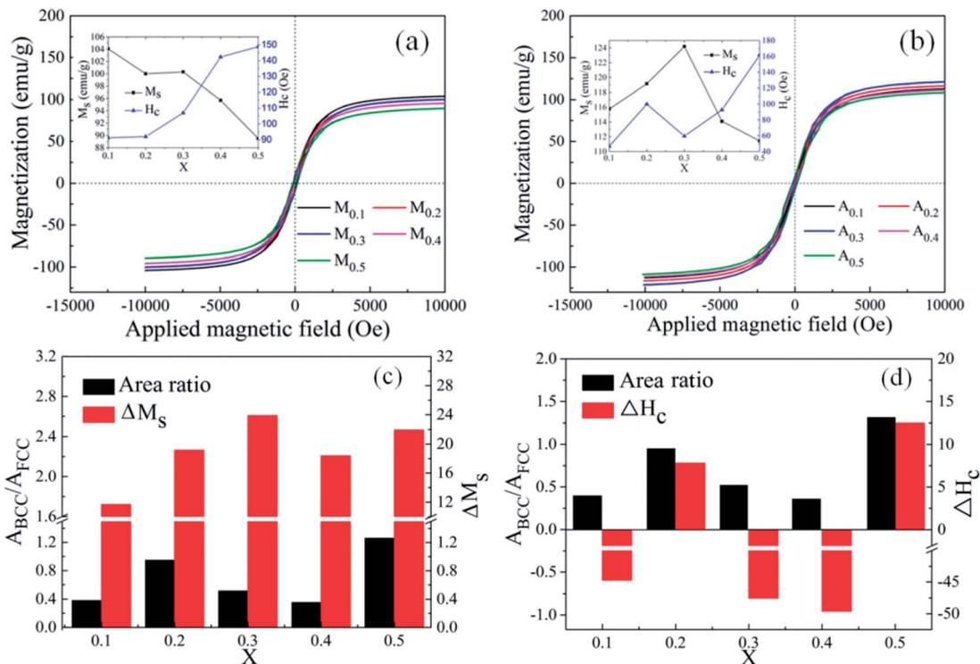
Fig. 4 Hysteresis loops of (a)  $M_{0.1-0.5}$  and (b)  $A_{0.1-0.5}$ , and the illustrations present the change in magnetic parameters ( $H_c$  and  $M_s$ ) of both kinds of alloy powders. (c–d) is the area ratio ( $A_{BCC}/A_{FCC}$ ),  $\Delta M_s$  ( $M_s(A_x) - M_s(M_x)$ ), and  $\Delta H_c$  ( $H_c(A_x) - H_c(M_x)$ ) for different alloy powders. Wherein  $X$  represents the molar amount of Si in  $FeCoNiSi_xAl_{0.4}$  alloy powders.
