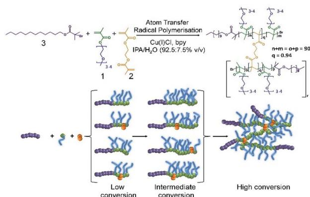
**Scheme 1** Synthesis of the branched copolymer emulsifier employing copper-catalysed ambient temperature ATRP of oligoethylene glycol monomethacrylate and ethylene glycol dimethacrylate in IPA/water. A dodecylbromoisobutyrate initiator was employed with a Cu(I)Cl/Bpy catalytic system (1/2) at an overall concentration of 44 v/v%.
