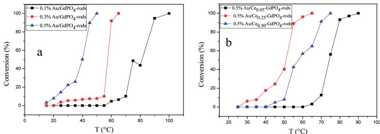
Fig. 14 CO conversion over Au/GdPO<sub>4</sub>-rods calcined 300 °C for 2 h with different gold loadings: 0.1%, 0.3%, 0.5% (a), and 0.5% Au/Ce-GdPO<sub>4</sub>-rods with the Ce contents of 5 at%, 25 at%, 50 at% (b).
