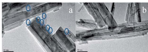
Fig. 5 TEM images of fresh 0.5% Au/Ce<sub>0.25</sub>-GdPO<sub>4</sub>-rods (a) and spent 0.5% Au/Ce<sub>0.25</sub>-GdPO<sub>4</sub>-rods calcined at 300 °C for 2 h.
