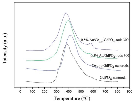
Fig. 9 CO<sub>2</sub>-TPD Profiles of the supports and Au supported catalysts.
