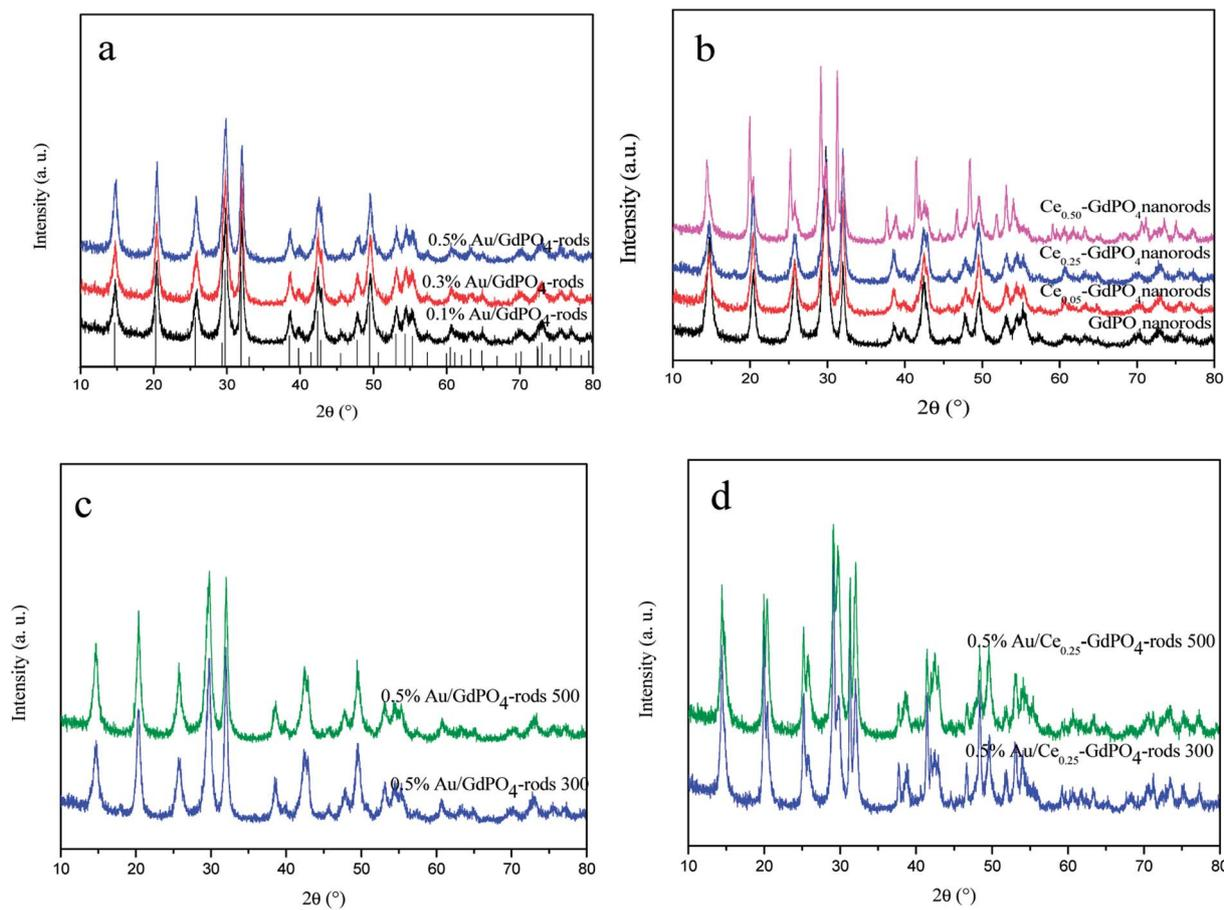
Fig. 1 XRD patterns of Au/GdPO<sub>4</sub>-rods with different Au contents (0.1%, 0.3%, 0.5%) calcined at 300 °C for 2 h (a), GdPO<sub>4</sub> and Ce-GdPO<sub>4</sub> supports (b), 0.5% Au/GdPO<sub>4</sub>-rods and 0.5% Au/Ce<sub>0.25</sub>-GdPO<sub>4</sub>-rods calcined at 500 °C for 2 h (c) and (d).
