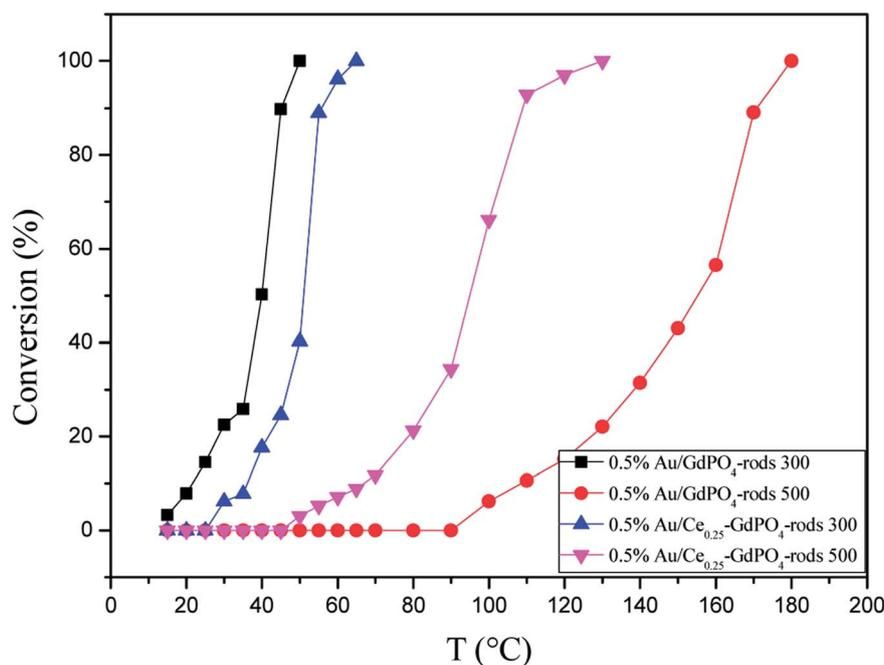
Fig. 15 CO conversion over 0.5% Au/GdPO<sub>4</sub>-rods and 0.5% Au/Ce<sub>0.25</sub>-GdPO<sub>4</sub>-rods calcined 300 °C or 500 °C for 2 h.
