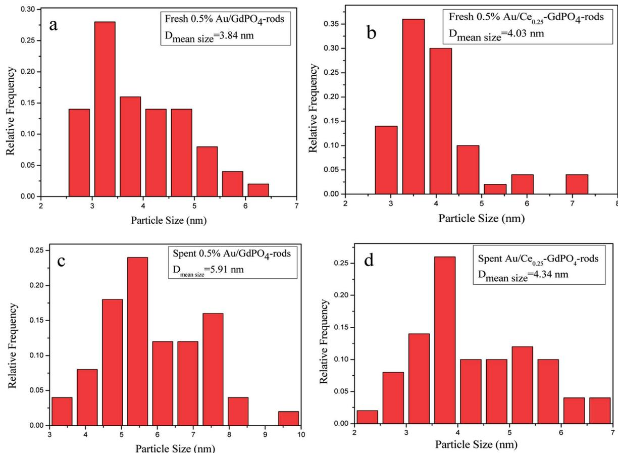
Fig. 6 Size distribution of catalysts (a) fresh 0.5% Au/GdPO<sub>4</sub>-rods, (b) fresh 0.5% Au/Ce<sub>0.25</sub>-GdPO<sub>4</sub>-rods, (c) spent 0.5% Au/GdPO<sub>4</sub>-rods, and (d) spent 0.5% Au/Ce<sub>0.25</sub>-GdPO<sub>4</sub>-rods.
