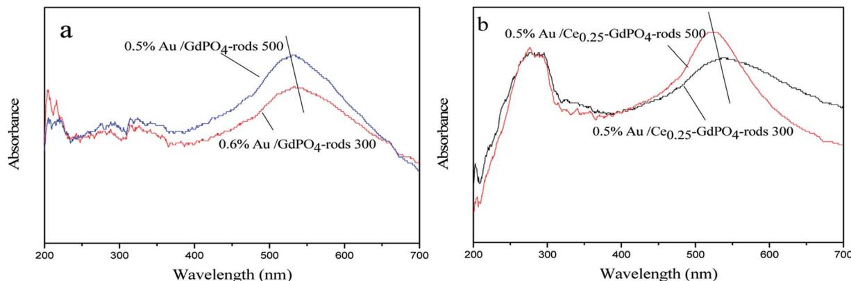
Fig. 13 UV-Vis spectra of 0.5% Au/GdPO<sub>4</sub>-rods (a) and 0.5% Au/Ce-GdPO<sub>4</sub>-rods (b) calcined at 300 and 500 °C for 2 h.
