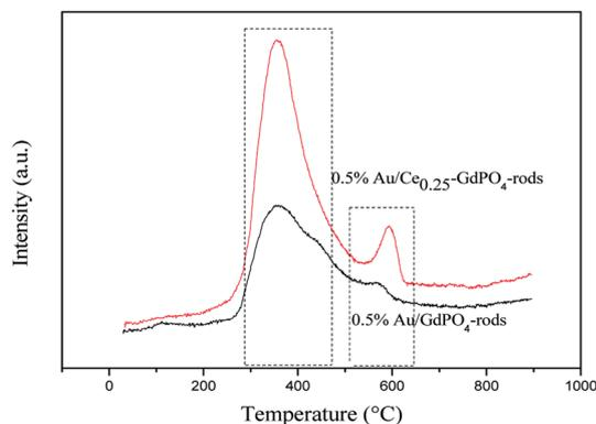
Fig. 10 CO-TPD profiles of the 0.5% Au/GdPO<sub>4</sub>-rods and 0.5% Au/Ce<sub>0.25</sub>-GdPO<sub>4</sub>-rods catalysts.
