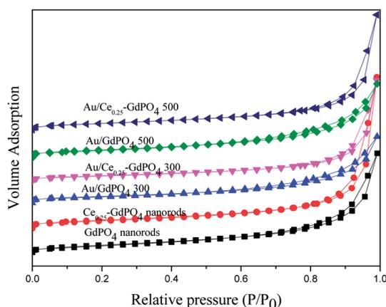
Fig. 2 Nitrogen adsorption-desorption isotherms of GdPO<sub>4</sub> nanorods, Ce<sub>0.25</sub>-GdPO<sub>4</sub> composites and the supported Au catalysts.
