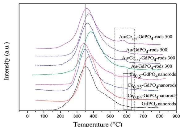
Fig. 8 O<sub>2</sub>-TPD profiles of GdPO<sub>4</sub> and Ce-GdPO<sub>4</sub> composites and Au supported catalysts.
