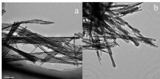
Fig. 3 TEM images of GdPO<sub>4</sub>-rods (a) and Ce<sub>0.25</sub>-GdPO<sub>4</sub>-rods (b).
