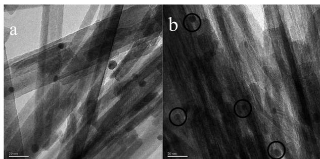
Fig. 7 TEM images of 0.5% Au/GdPO<sub>4</sub>-rods (a) and 0.5% Au/Ce<sub>0.25</sub>-GdPO<sub>4</sub>-rods (b) calcined at 500 °C for 2 h.
