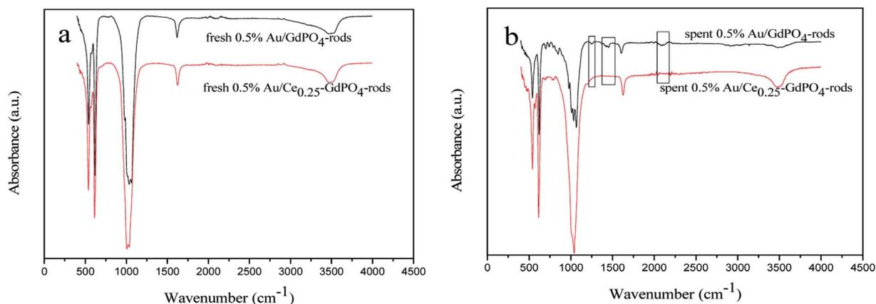
Fig. 12 FT-IR spectra of 0.5% Au/GdPO<sub>4</sub>-rods (a) and 0.5% Au/Ce<sub>0.25</sub>-GdPO<sub>4</sub>-rods (b) calcined at 300 °C for 2 h.
