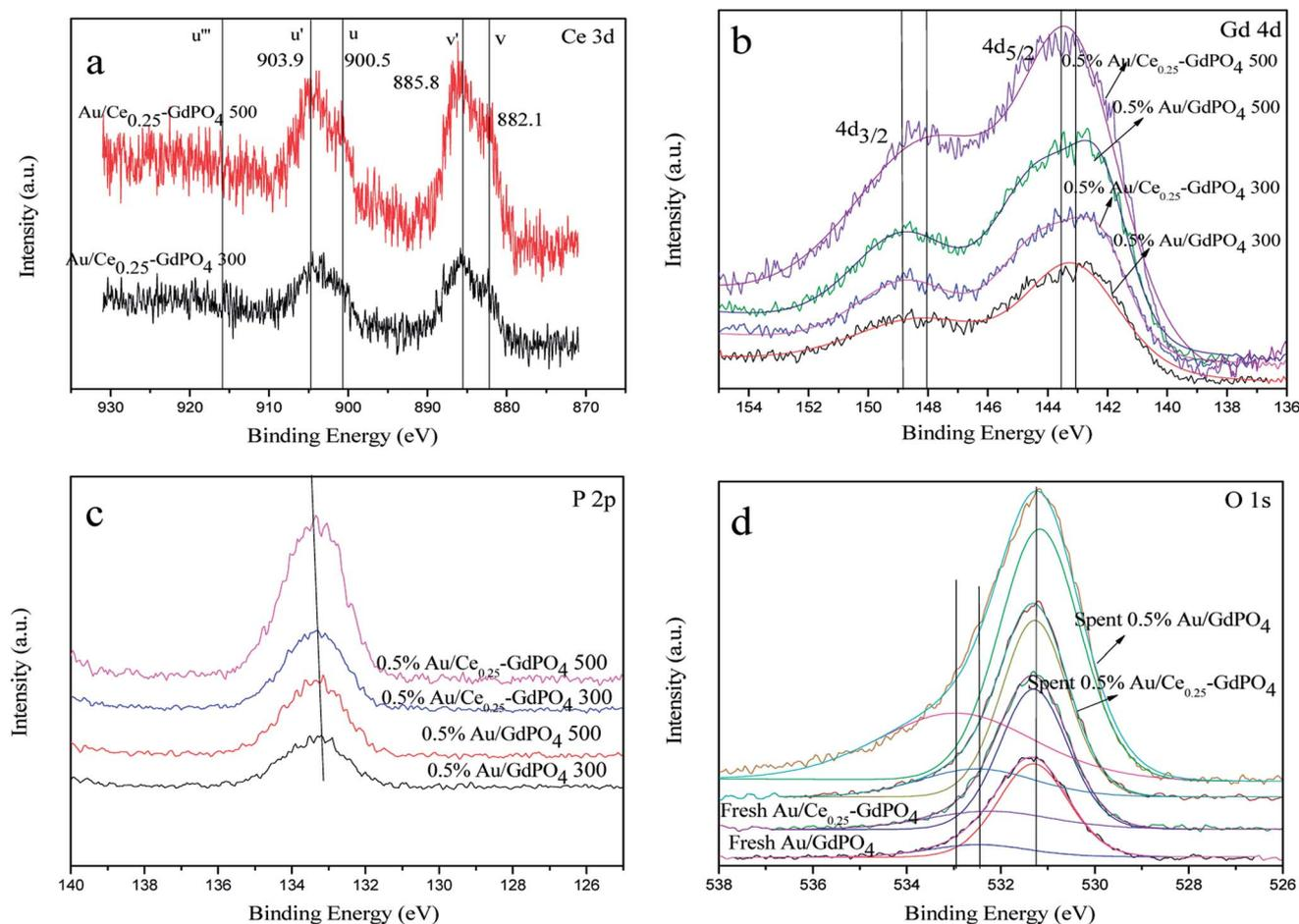
Fig. 11 XPS spectra over fresh and spent 0.5% Au/GdPO<sub>4</sub>-rods and 0.5% Au/Ce<sub>0.25</sub>-GdPO<sub>4</sub>-rods calcined at 300 °C or 500 °C for 2 h of Ce 3d (a), Gd 4d (b), P 2p (c), O 1s (d).
