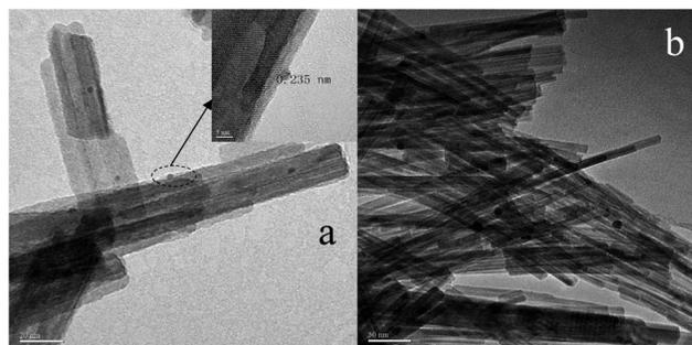
Fig. 4 TEM images of fresh 0.5% Au/GdPO<sub>4</sub>-rods (a) and spent 0.5% Au/GdPO<sub>4</sub>-rods calcined at 300 for 2 h.
