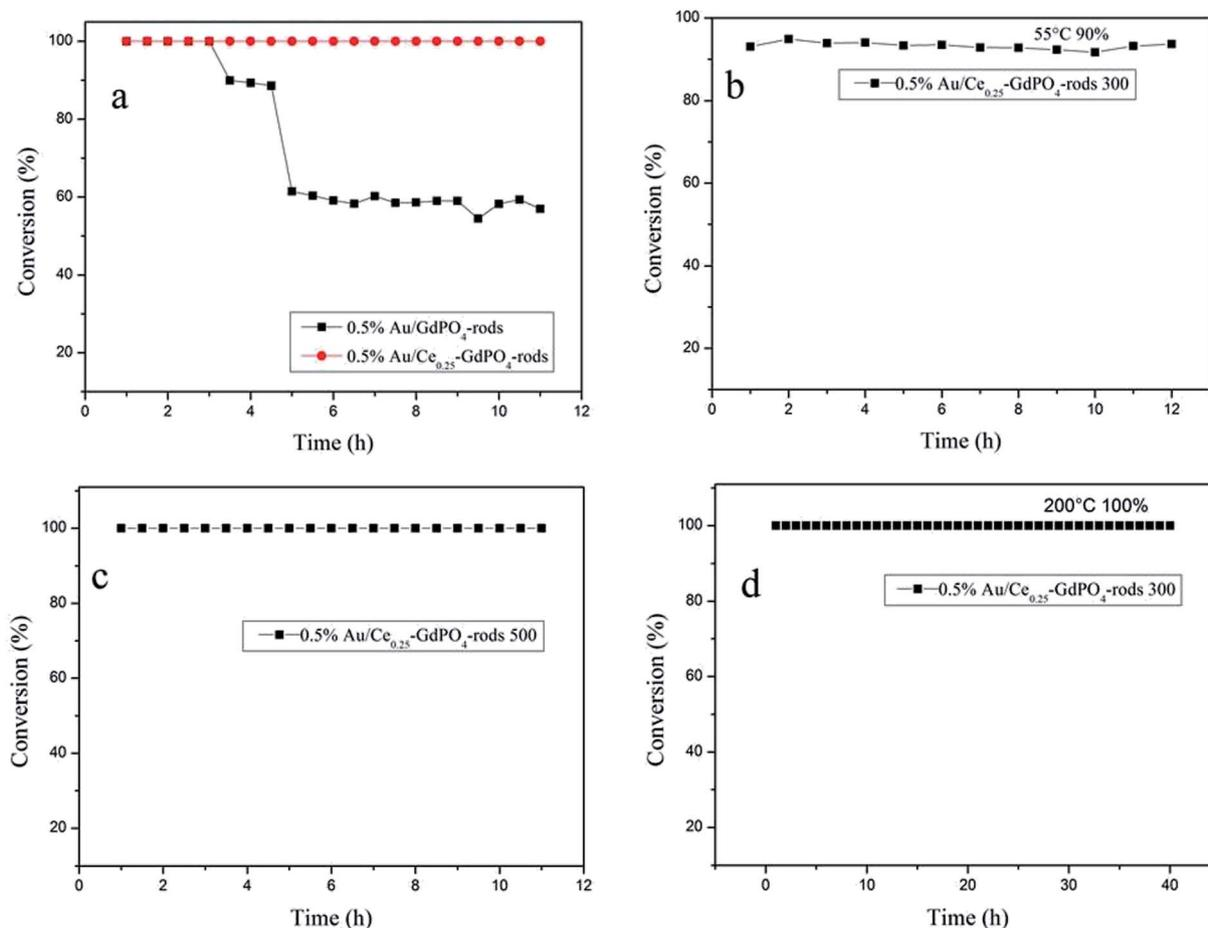
Fig. 16 The stability for the CO oxidation of 0.5% Au/GdPO<sub>4</sub>-rods, 0.5% Au/Ce<sub>0.25</sub>-GdPO<sub>4</sub>-rods ( $T_{100\%} = 50$  °C and 65 °C, respectively) (a), 0.5% Au/Ce<sub>0.25</sub>-GdPO<sub>4</sub>-rods,  $T_{90\%} = 55$  °C calcined at 300 °C for 2 h (b), 0.5% Au/Ce<sub>0.25</sub>-GdPO<sub>4</sub>-rods calcined at 500 °C,  $T_{100\%} = 130$  °C (c), 0.5% Au/Ce<sub>0.25</sub>-GdPO<sub>4</sub>-rods calcined at 300 °C, reaction temperature: 200 °C (d).
