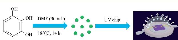
Fig. 1 A schematic of CDs synthesis and their application in white LED.
