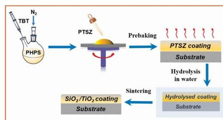
Fig. 1 A schematic illustration of the SiO<sub>2</sub>/TiO<sub>2</sub> coating preparation.
