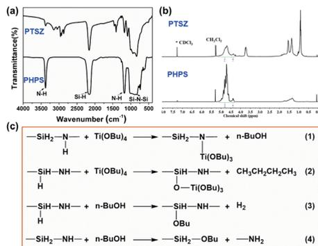
Fig. 2 The chemical structures of PHPS and PTSZ: (a) FT-IR spectra; and (b) <sup>1</sup>H-NMR spectra. (c) Possible reactions between PHPS and TBT.
