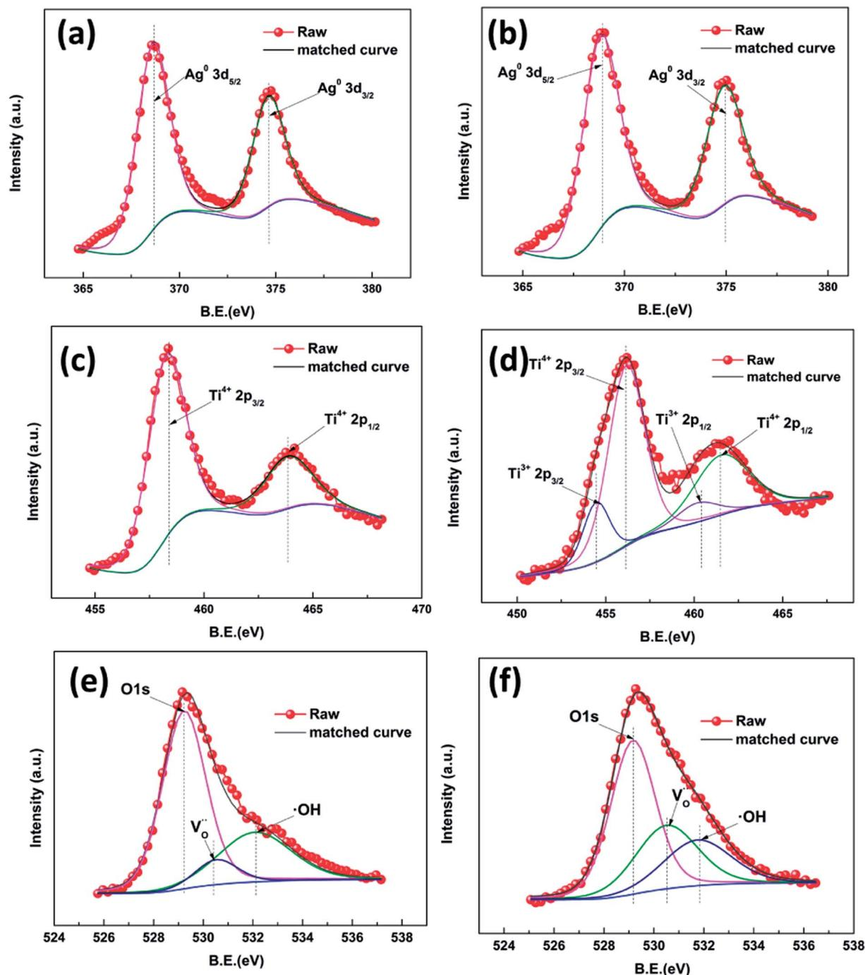
Fig. 5 High resolution XPS spectra of Ag 3d of different samples: AP1 (a) and ACP1 (b); Ti 2p: AP1 (c) and ACP1 (d); O 1s: AP1 (e) and ACP1 (f).
