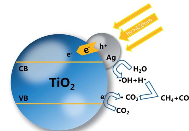
Scheme 2 Schematic of mechanism for photocatalytic process of TiO<sub>2</sub> decorated with AgNPs and surface self-doping.
