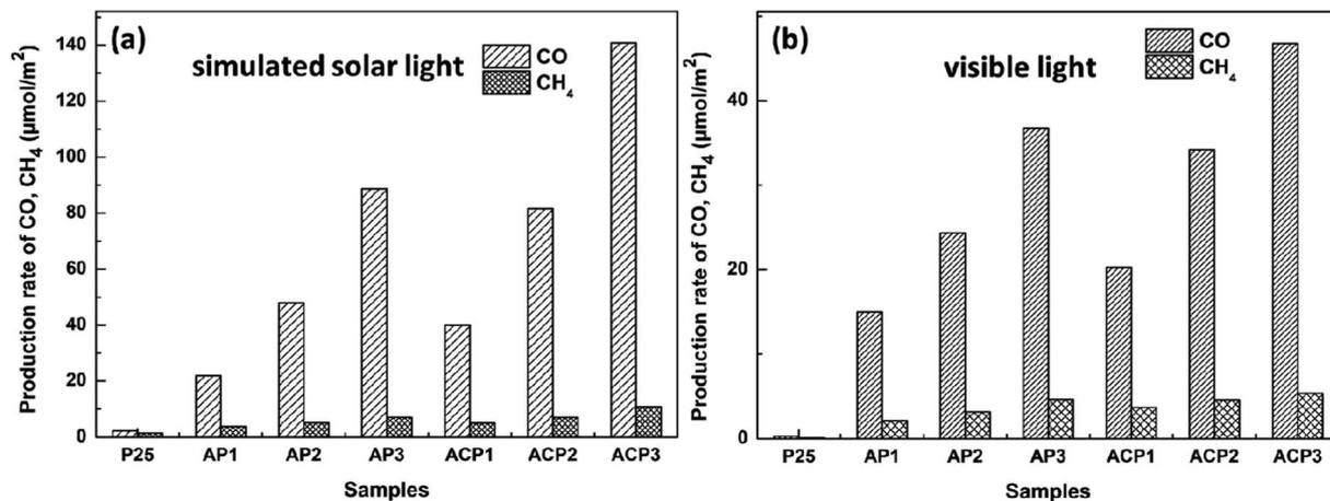
Fig. 7 Evolution of CO and CH<sub>4</sub> yields of different samples under simulated solar light (a) and visible light (b).
