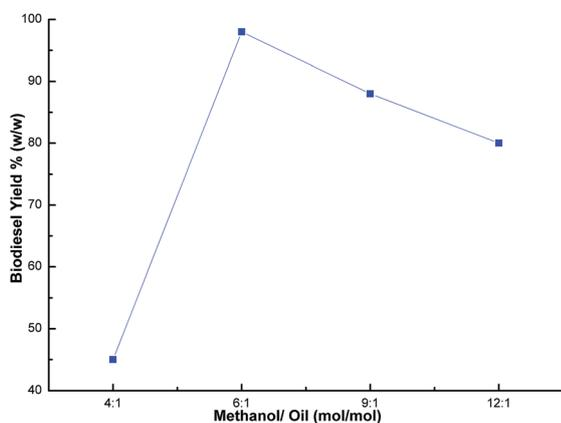
Fig. 9 Effect of methanol/oil ratio on biodiesel yield.
