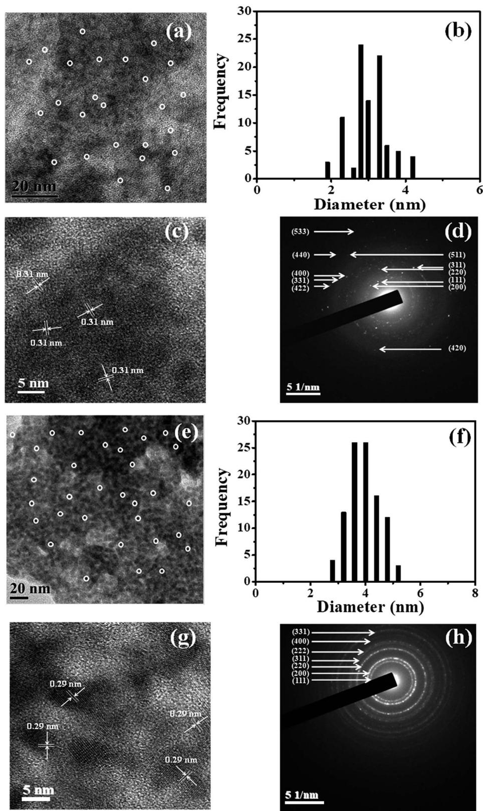
Fig. 3 The TEM images, size distributions, HRTEM images and SAED patterns of the Zn(Tb)S and post-synthetically modified Zn(Tb)S nanoparticles with  $[\text{Zn(Tb)S}] : [\text{Pb}^{2+}] = 1 : 1$  are shown in panels (a) and (e), (b) and (f), (c) and (g), and (d) and (h), respectively.
