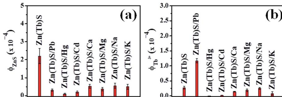
Fig. 11 The trend in the broad and sharp emission of the ZnS nanoparticles (panel a) and  $\text{Tb}^{3+}$  (panel b), respectively, are shown for cases where the Zn(Tb)S nanoparticles were post-synthetically treated with  $\text{M}^{n+}$ , with  $[\text{Zn}(\text{Tb})\text{S}] : [\text{M}^{n+}] = 1 : 10^{-2}$ . The values reported are average and standard deviation from two independent measurements.
