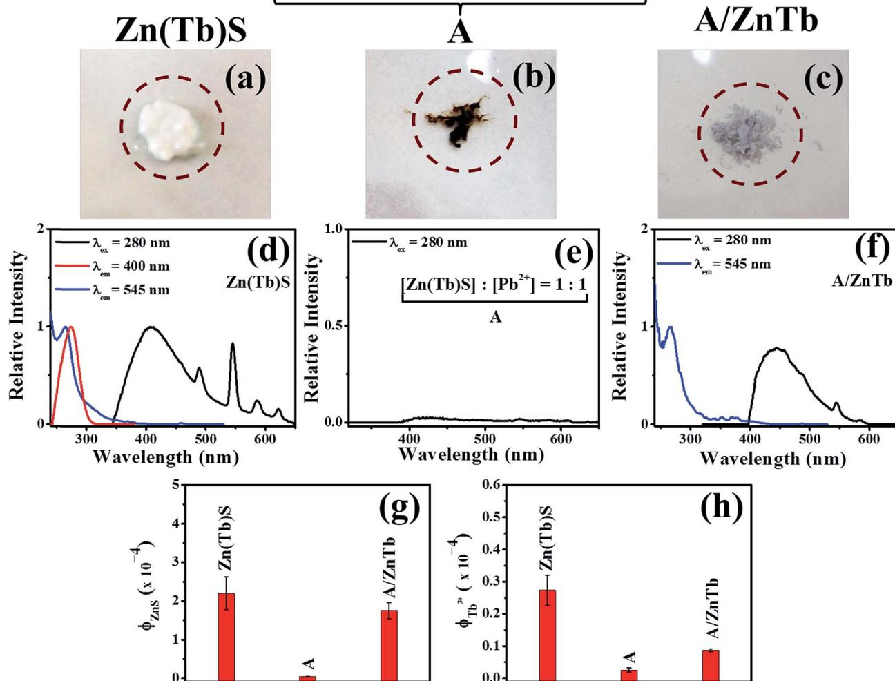
Fig. 8 Images of initial Zn(Tb)S, [Zn(Tb)S] : [Pb<sup>2+</sup>] = 1 : 1 (A), and A/ZnTb are shown in panels (a)–(c). The relevant photoluminescence excitation and emission spectra are shown in panels (d)–(f), with the trends in emission quantum yields shown in panels (g) and (h).
