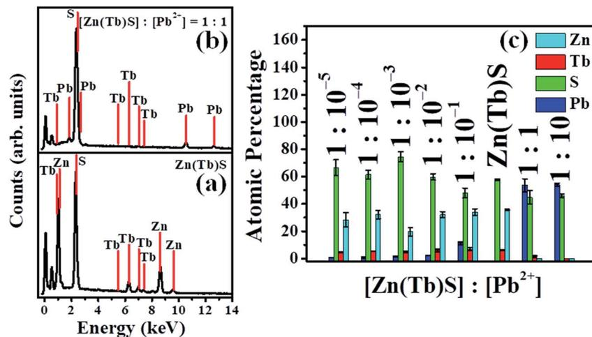
Fig. 5 Panels (a) and (b) show the EDS spectra of the Zn(Tb)S and post-synthetically modified Zn(Tb)S nanoparticles with  $[\text{Zn(Tb)S}] : [\text{Pb}^{2+}] = 1 : 1$ , respectively. Panel (c) shows the elemental composition of the Zn(Tb)S nanoparticles with various  $\text{Pb}^{2+}$  concentrations that have been added post-synthetically.
