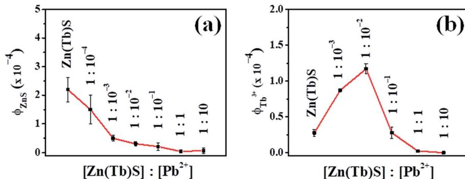
Fig. 12 The relative emission of the broad ZnS and sharp Tb<sup>3+</sup> in the post-synthetically modified Zn(Tb)S nanoparticles as a function of [Pb<sup>2+</sup>] is shown. The lines on the curves are a visual representation indicating the deviation from linearity.
