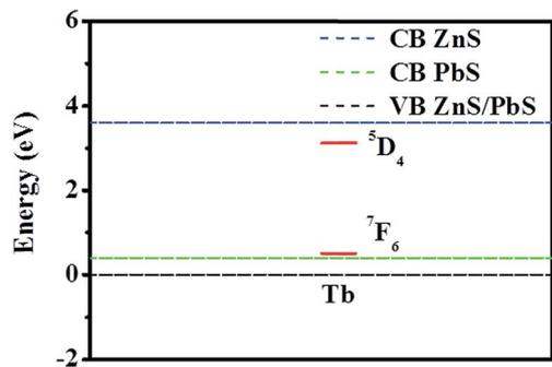
Fig. 9 Relative energy level positions of the  $\text{Tb}^{3+}$  ground and luminescent energy levels are shown with respect to the valence and conduction bands of the host materials. In constructing the energy level schematic, the bulk band gap values of the respective materials have been considered.
