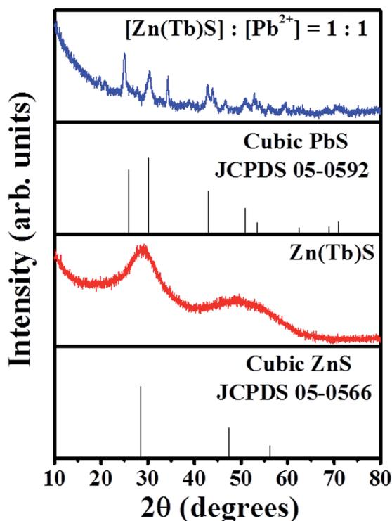
Fig. 2 XRD profiles of the Zn(Tb)S nanoparticles and the sample with [Zn(Tb)S] : [Pb<sup>2+</sup>] = 1 : 1 are shown.
