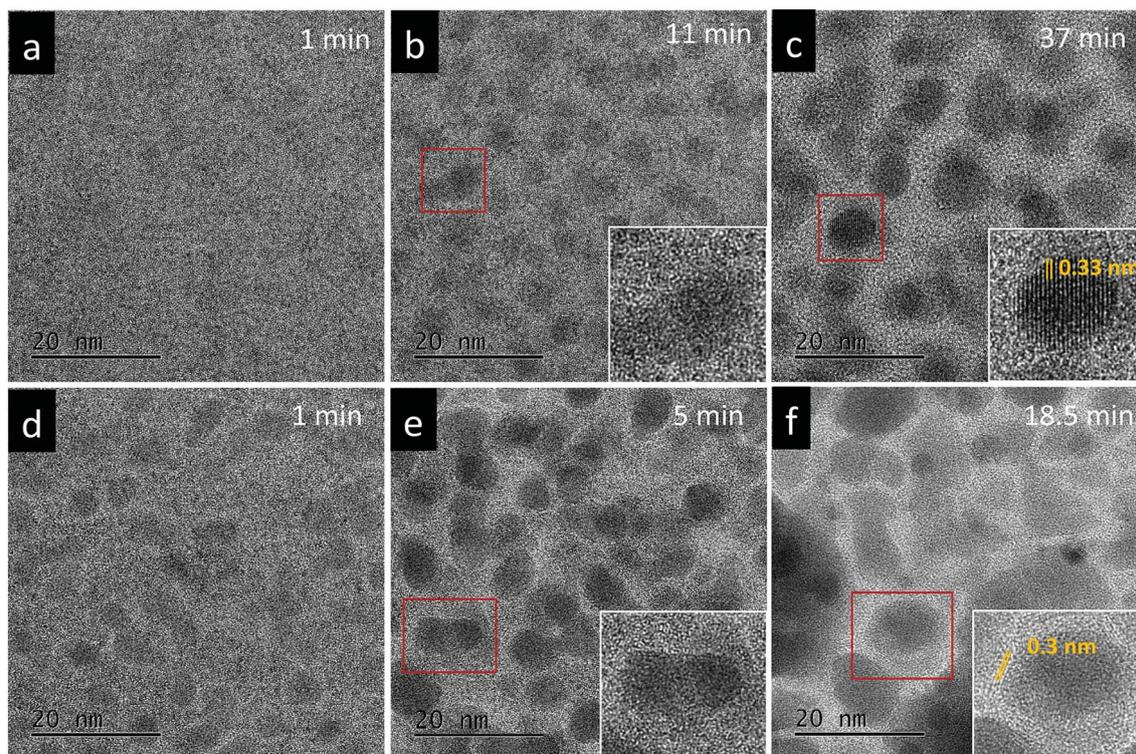
Fig. 2 Time sequential TEM images of the amorphous bismuth ferrite films under thermal heating at (a–c) 100 °C, and (d–f) 300 °C. The electron dose rates used are  $2.7 \times 10^3 \text{ e} (\text{\AA}^2 \text{ s}^{-1})$  and  $2.6 \times 10^3 \text{ e} (\text{\AA}^2 \text{ s}^{-1})$  for (a–c) and (d–f), respectively. Selected particles (marked by red squares) are enlarged as shown in the inserted HRTEM images to show the crystallization process.
