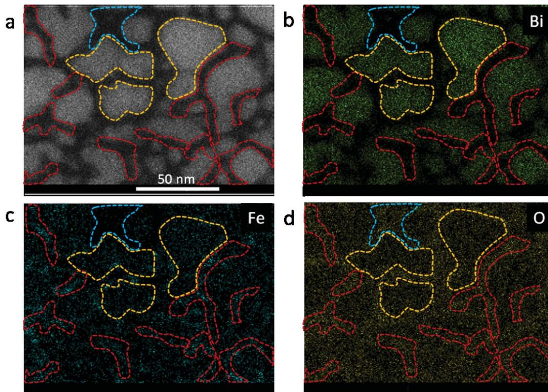
**Fig. 3** EDS elemental mapping of bismuth ferrite film performed after the sample was heated to 300 °C. (a) HAADF-STEM image, (b) Bi, (c) Fe and (d) O elemental distributions. The yellow dashed lines enclose Bi-enriched region, the red lines Fe and O en-riched area, and the blue lines shows the void area. The electron dose rate used is  $3 \times 10^3 \text{ e} (\text{Å}^2 \text{ s})^{-1}$ .
