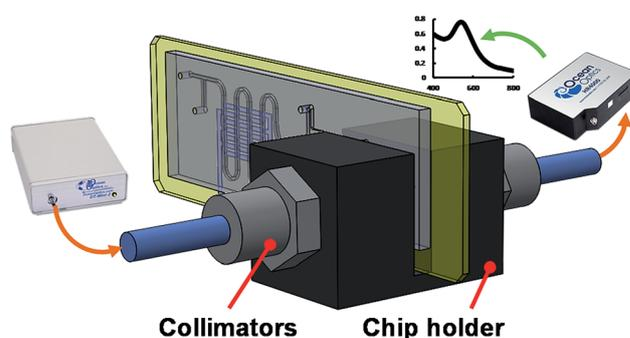
Fig. 6 The experimental setup for UV-Vis detecting the Hg<sup>2+</sup> reaction with AuNPs in the microchip.
