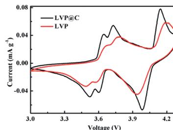
Fig. 5 CV profiles of LVP@C NCs and LVP NCs at a scanning rate of 0.1 mV s<sup>-1</sup> from 3.0 to 4.3 V.
