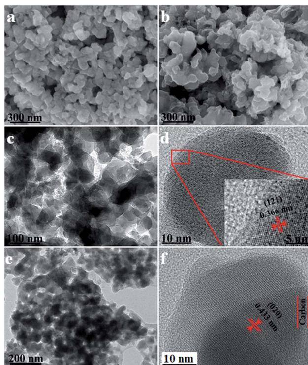
Fig. 3 SEM images of (a) LVP and (b) LVP@C, TEM images of (c) LVP and (e) LVP@C, and HRTEM images of (d) LVP and (f) LVP@C.
