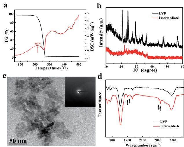
Fig. 2 (a) DSC curves of vanadium(III) acetylacetonate at  $10\text{ }^{\circ}\text{C min}^{-1}$  under nitrogen. (b) XRD patterns of the intermediate and LVP. (c) TEM image of the intermediate and the corresponding SAED pattern (inset). (d) FT-IR spectra of the intermediate and LVP.
