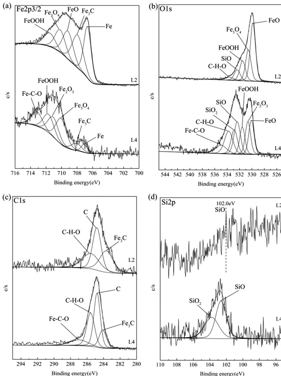
Fig. 8 XPS analysis results of the rubbing surfaces for 150SN with attapulgite powder (L2) and attapulgite/La<sub>2</sub>O<sub>3</sub> nanocomposite (L4): (a) Fe2p<sub>3/2</sub>; (b) O1s; (c) C1s; (d) Si2p.
