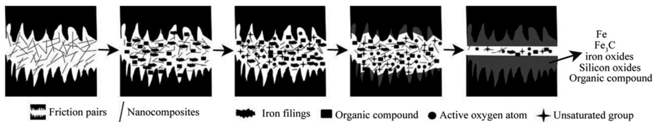
Fig. 10 Formation mechanism of the tribofilm generated by attapulgite/La<sub>2</sub>O<sub>3</sub> nanocomposite.
