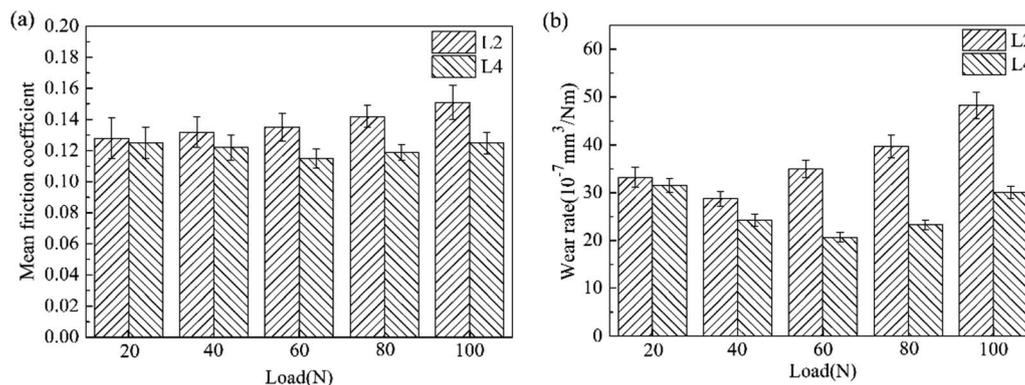
Fig. 11 The effect of load on the tribological properties of lubricants.
