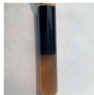
Fig. 6 Photograph of crude-oil-in-simulated formation water middle phase microemulsion taken after 3 weeks of settling 45 °C.
