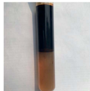
Fig. 6 Photograph of crude-oil-in-simulated formation water middle phase microemulsion taken after 3 weeks of settling 45\text{ }^{\circ}\text{C} .
