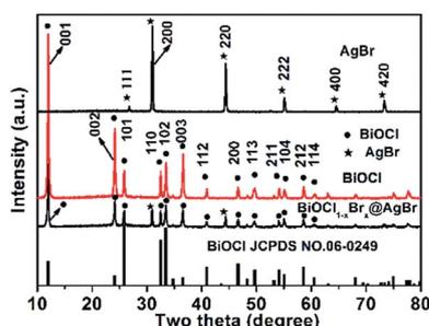
Fig. 1 XRD diffraction patterns of AgBr, BiOCl and BiOCl<sub>1-x</sub>Br<sub>x</sub>@AgBr.
