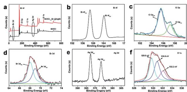
Fig. 2 (a) XPS survey spectra of BiOCl<sub>1-x</sub>Br<sub>x</sub>@AgBr and BiOCl and (b-f) XPS spectra of the Bi, Cl, Br, Ag and O elements in BiOCl<sub>1-x</sub>Br<sub>x</sub>@AgBr.
