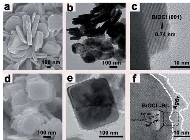
Fig. 3 (a) SEM images of BiOCl, (b and c) TEM and HRTEM images of BiOCl, (d) SEM image of BiOCl<sub>1-x</sub>Br<sub>x</sub>@AgBr and (e and f) TEM and HRTEM images of BiOCl<sub>1-x</sub>Br<sub>x</sub>@AgBr.
