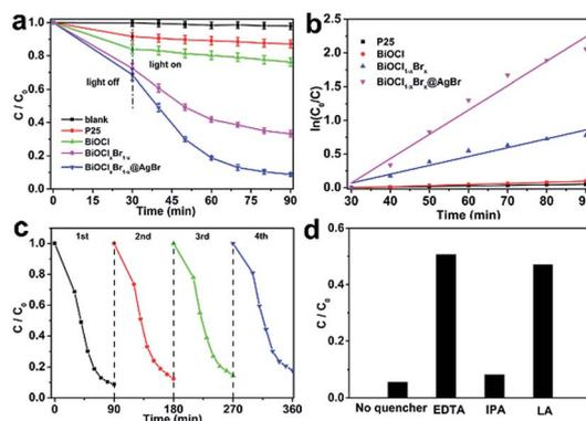
Fig. 7 (a) Photocatalytic activities of different samples under visible light irradiation ( $\lambda > 420 \text{ nm}$ ), (b) kinetic fit for degradation of dyes with different samples, (c) cycling runs of  $\text{BiOCl}_{1-x}\text{Br}_x@\text{AgBr}$  for degradation of Reactive Blue KN-R under visible light and (d) degradation rate of Reactive Blue KN-R over  $\text{BiOCl}_{1-x}\text{Br}_x@\text{AgBr}$  after adding different scavengers.
