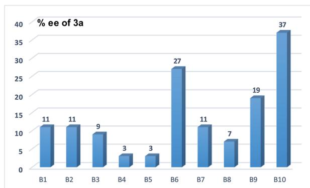
Fig. 1 The effect of base (B1–B10) on the enantioselectivity in the Pd-catalyzed tandem allylic substitution/cyclization: B1 ( $\text{K}_2\text{CO}_3$ ), B2 ( $\text{KHCO}_3$ ), B3 ( $\text{K}_3\text{PO}_4$ ), B4 (KF), B5 ( $\text{Na}_2\text{CO}_3$ ), B6 ( $\text{NaHCO}_3$ ), B7 ( $\text{Cs}_2\text{CO}_3$ ), B8 (DBU), B9 ( $\text{Et}_3\text{N}$ ) and B10 (DIPEA).
