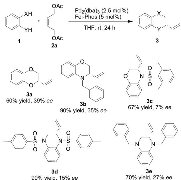
**Scheme 2** Fei-Phos ligand-controlled palladium-catalyzed tandem allylic alkylation of different 1,2-bifunctional nucleophiles **1** with the (*Z*)-but-2-ene-1,4-diol derived allylic acetate **2a**: a representative substrate scope.
