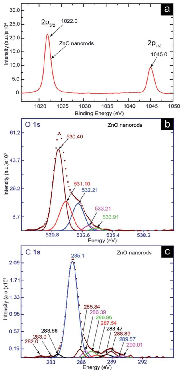
Fig. 6 XPS spectra of ZnO nanorods. (a) ZnO 2p<sub>3/2</sub> 2p<sub>1/2</sub>, (b) ZnO O 1s, and (c) C 1s core level XPS spectra.
