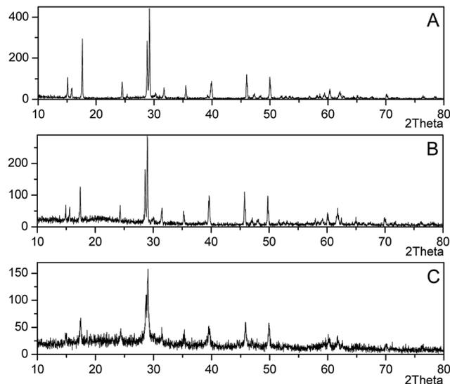
Fig. 3 XRD patterns of jarosite and fungal induced mineral (pH 2.5, 11<sup>th</sup> day): (A) Jarosite XRD standard pattern (PDF#22-0827); (B) XRD pattern of mineral formed in control experiments without cells; (C) XRD pattern of mineral induced by *P. lilacinum* Y3.
