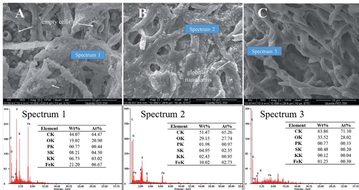
Fig. 6 SEM micrographs showed the effect of EPS on biomineralization (pH 2.5, 2<sup>nd</sup> day): (A) autoclaved method; (B) ultrasonic method; (C) comprehensive method.
