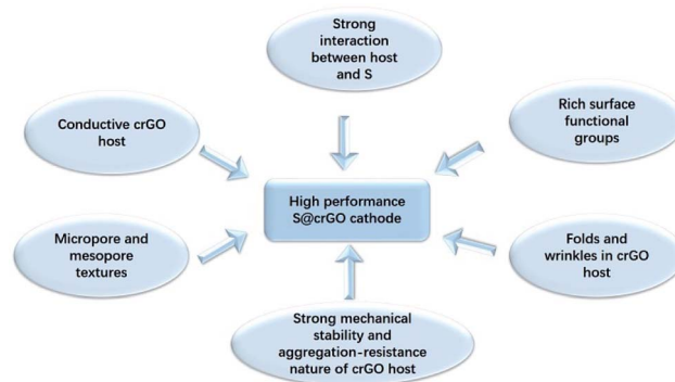
Scheme 1 Reasons for the high performance of S@crGO cathode for Li–S batteries.
