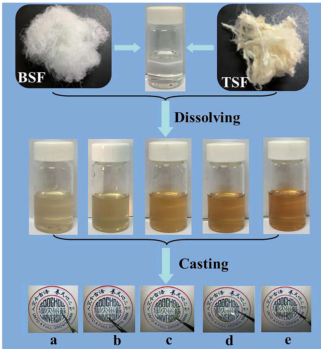
Fig. 1 Preparation process of BSF/TSF blend films with various blend ratios. (a) BSF, (b) 3/1, (c) 1/1, (d) 1/3, (e) TSF.
