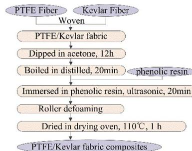
Fig. 2 Manufacturing process of hybrid PTFE/Kevlar fabric composites.
