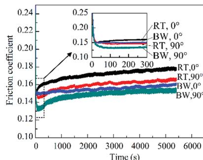
Fig. 5 Variations of friction coefficient with sliding time for RT and BW along orientations of 0° and 90° (load 8 MPa, reciprocating frequency 5 Hz).
