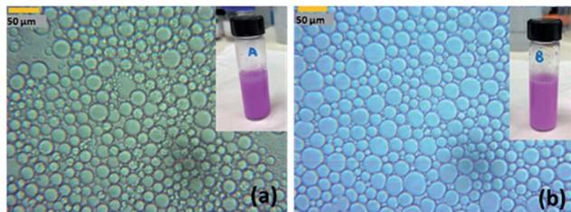
**Fig. 3** Optical microscopic (40×) and camera images taken after fresh preparation of emulsions *via* ultrasonic homogenization. (a) **9a**/water/*n*-decane; (b) **11**/water/*n*-decane (both with rhodamine dye for better visualization).
